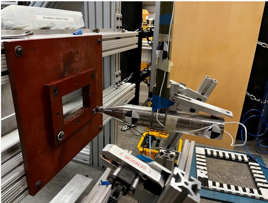
Figure 2.2: Pendulum Impactor System Set-up
