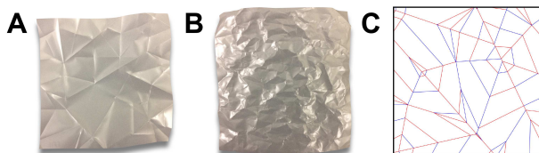
FIG. 1. Examples of crease networks: (A) A 10 cm \times 10 cm sheet of Mylar that has undergone a succession of rigid flat-folds. (B) A sheet of Mylar that has been crumpled. (C) A simulated rigid flat-folded sheet. The sheet has been folded 13 times. Ridges are colored red, and valleys are blue.
