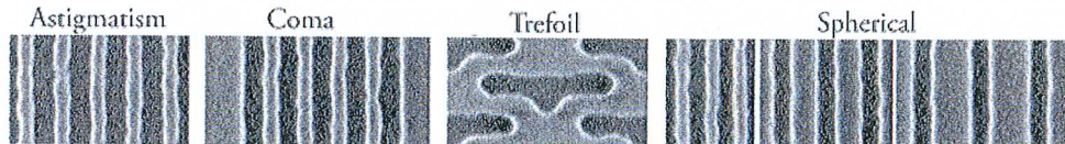
Figure 7. Examples of the CD-SEM micrographs used for CD measurements to extract the NXE:3100 aberrated wavefront.
