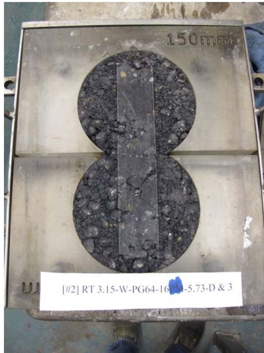
Figure C.5: HWTT result for PG 64-16 25% RAP, 1.2% lime (set #1 rt.) after 40,000 passes.
