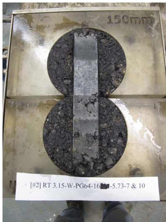
Figure C.8: HWTT result for PG 64-16 25% RAP, 1.2% lime (set #2, lt.) after 40,000 passes.
