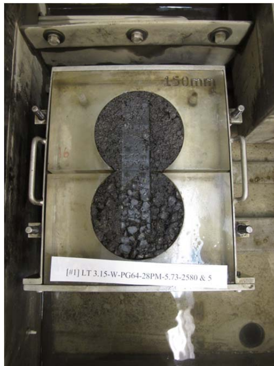
Figure C.2: HWTT result for PG 64-28PM 15% RAP, 1.2% lime (set #1, lt.) after 40,000 passes.
