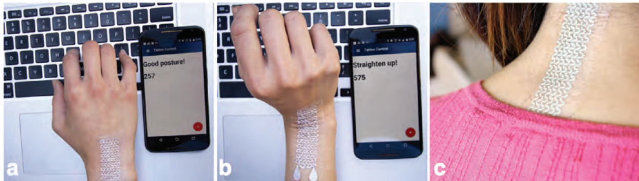
Figure 6.13: Strain gauge for body position sensing. a) The strain gauge reading indicates that the user’s wrist is in a correct typing position. b) The strain gauge reading indicates that the user’s wrist is not at a correct posture, which causes the mobile phone to send a warning message. c) The strain gauge can also be worn on other body positions, such as the neck and back, to detect movement and posture.
