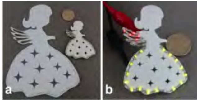
Figure 4.8: ShrinkyCircuit cut with a low-cost vinyl cutter. a) Polymer substrate prior to shrinking. b) ShrinkyCircuit under operation.
