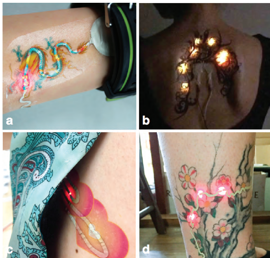
Figure 6.9: Example of Skintillates tattoo displays. a) a dragon Skintillates display is powered by the watch and could serve as a point-light display, b) a back Skintillates tattoo that flashes with the beat of the music around the wearer, c) a private Skintillates tattoo flashing according to ECG signals, d) a Skintillates tattoo without a printed art layer decorates an existing permanent tattoo
