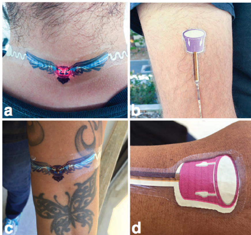
Figure 6.14: Representative Pictures of Skintillates Devices in User Study. Participants were free to apply the Skintillate tattoo on any body location. Example applied body locations include a) neck, and b) arm. c) Skintillate LED displays used in the study utilize small 0603 LED parts, which allows the Skintillate tattoo to retain its conformal profile. d) Skintillates resistive sensor used in the study worn on arm.
