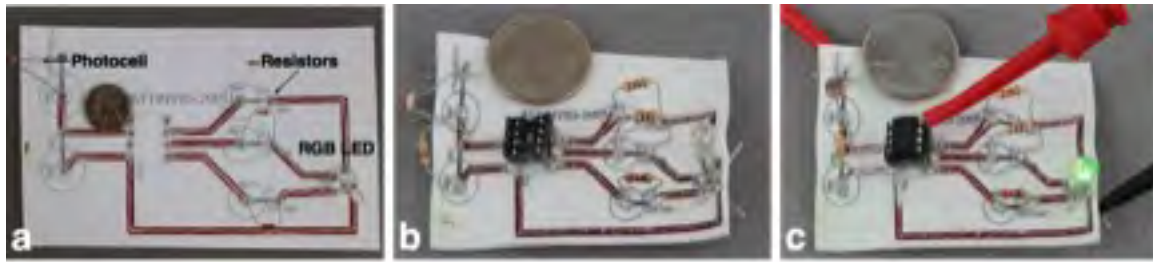
Figure 4.7: A ShrinkyCircuit designed using Eagle PCB software. a) Electronic components loaded on a circuit printed on polymer sheet with inkjet printer. The electrical connections are traced with a connective pen. c) IC holder is inserted into the shrunk circuit after the polymer substrate is heated. d) The ShrinkyCircuit under operation.
