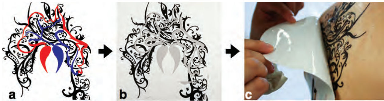
Figure 6.5: Skintillates fabrication process work flow. a) the art layer (in black) and the electrical traces (in red and blue) are designed in a standard design program, b) the art layer (in black) is inkjet printed and the conductive layer (in silver) screen-printed on the tattoo substrate, and c) the Skintillate device is applied on skin and released from the paper backing.
