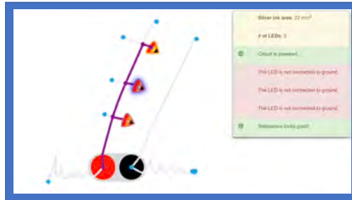
Figure 7.8: Validation tool checks for errors in the electrical design before the user fabricate the circuit. This figure shows
