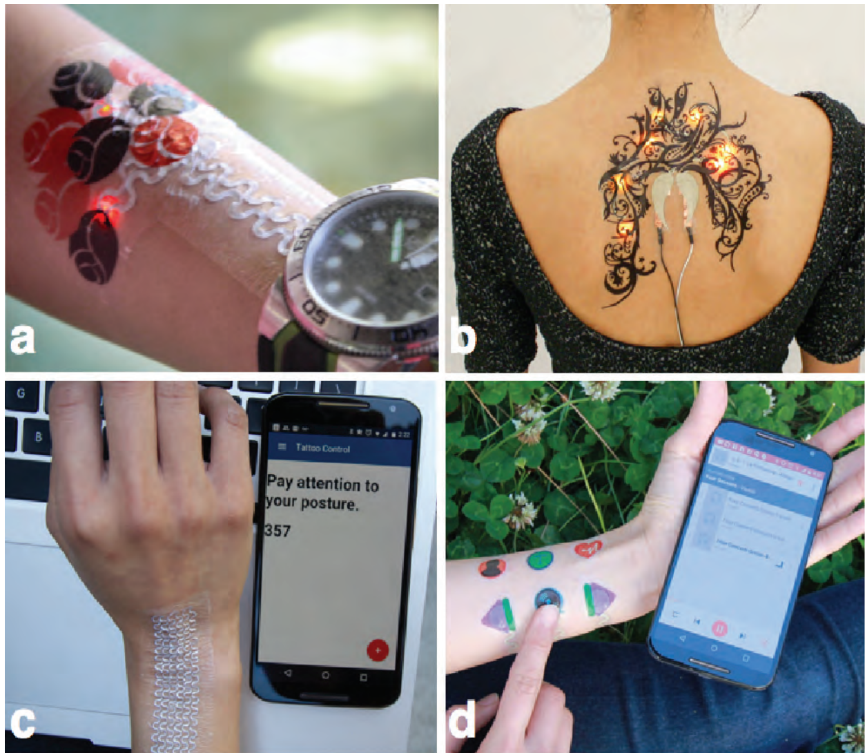
Figure 6.3: Skintillates is a class of temporary tattoo electronics that can be fabricated using an accessible process. a) A point-light display, b) A back tattoo LED display that flashes with music, c) A strain gauge that detects body position, d) capacitive buttons for mobile device control
