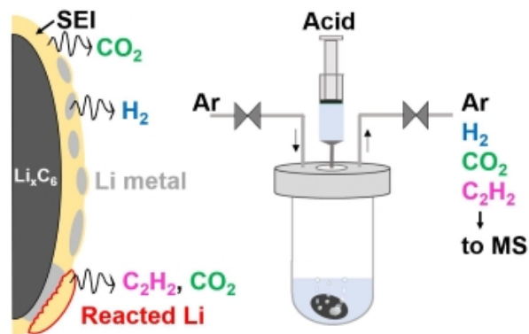
Figure 3.1: MST Schematic. Left side: Common gases evolved during MST. SEI components are primarily solid carbonates (e.g., lithium ethylene dicarbonate), which evolve \text{CO}_2 upon immersion in acid. Li metal is known to form lithium acetylide ( \text{Li}_2\text{C}_2 ) in small quantities when reacted with other carbonate-containing SEI components. Upon exposure to water, \text{Li}_2\text{C}_2 releases acetylene gas ( \text{C}_2\text{H}_2 ). Li metal is highly reactive with water and evolves \text{H}_2 gas. Right panel: an image of the MST titration vessel. An electrode is sealed in the vessel and acid is injected. Gases are carried to a mass spectrometer where they are quantified using an in-line gas handling unit.
