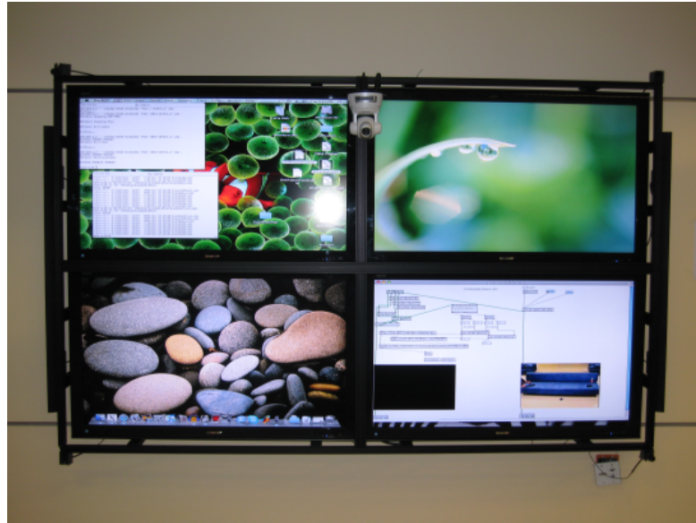
Figure 1.1: Frontal view of TAC display unit. PTZ camera and four of the seven total microphone are visible.
