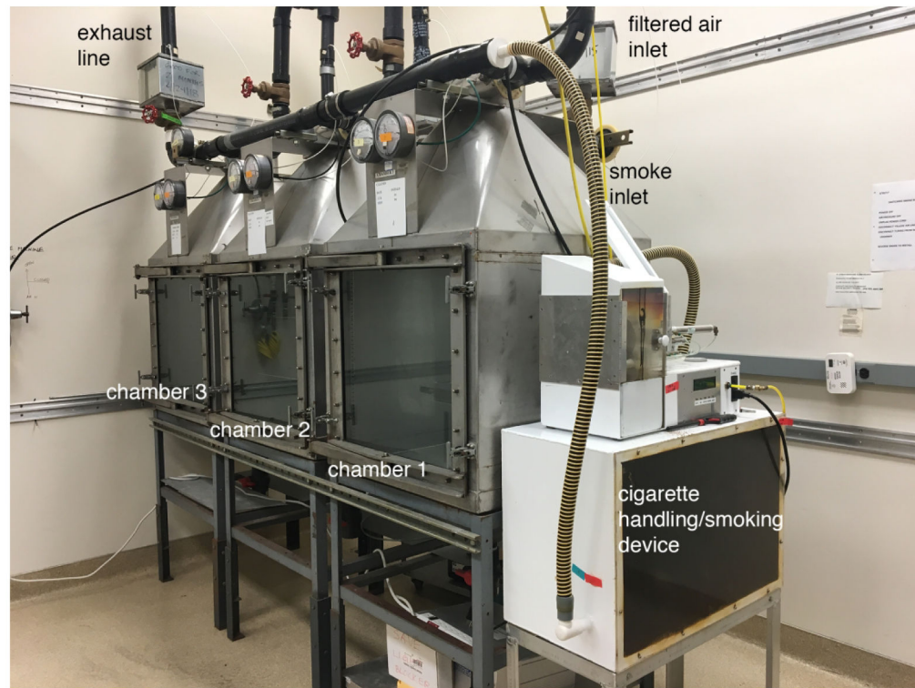
Figure 1. Tobacco smoke exposure chambers.
