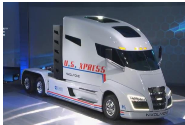
Figure 14. Nikola One hydrogen fuel cell truck [Source: nikolamotor.com]
