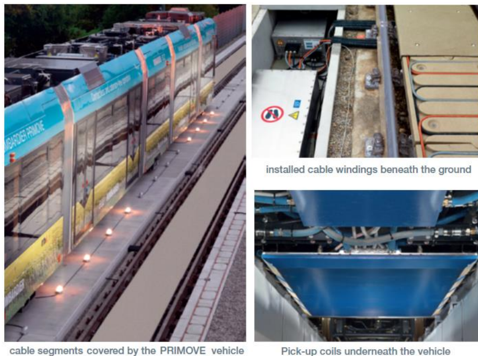
Figure 8. Bombardier PRIMOVE dynamic inductive charging light rail [Source: http://primove.bombardier.com ]
