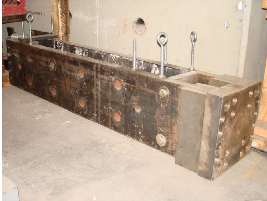
Figure 4-8 Photograph of lateral load transfer assembly
