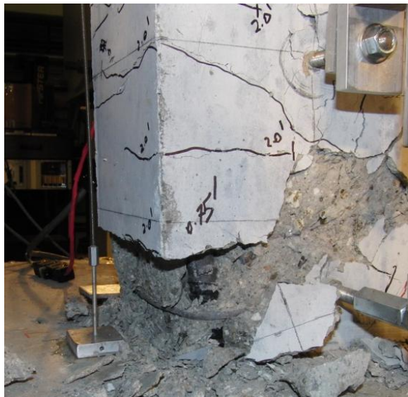
Figure 6-25 RW-A15-P10-S78: North and south wall boundaries at 3.0% drift after first cycle
