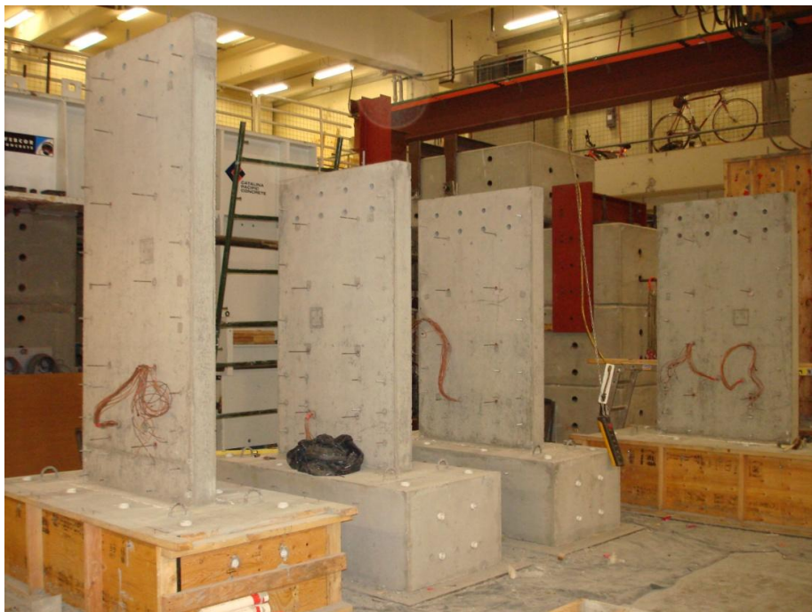
Figure 5-16 Specimens after formwork removal
