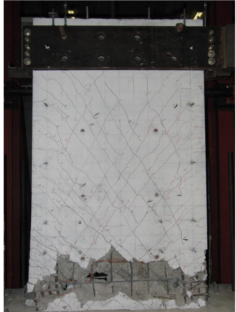
Figure A-17 Crack patterns for RW-A15-P10-S78: (a) 2.0% Drift, and (b) At end of test
