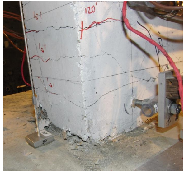
Figure 6-23 RW-A15-P10-S78: North and south wall boundaries at 1.5% drift after third cycle
