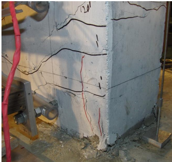
Figure 6-23 RW-A15-P10-S78: North and south wall boundaries at 1.5% drift after third cycle
