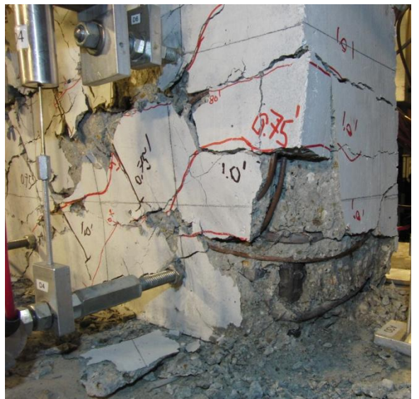
Figure 6-25 RW-A15-P10-S78: North and south wall boundaries at 3.0% drift after first cycle
