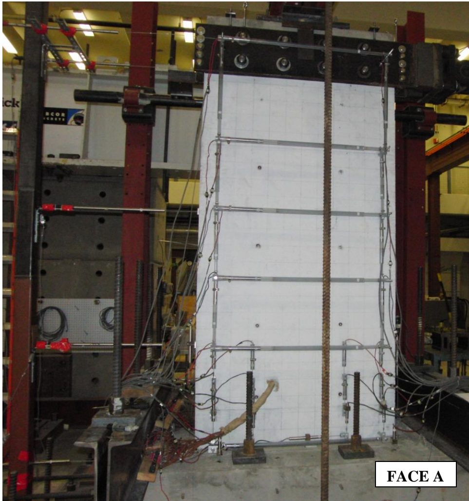
Figure 5-2 Photograph of LVDT configuration for specimens with aspect ratio 2.0
