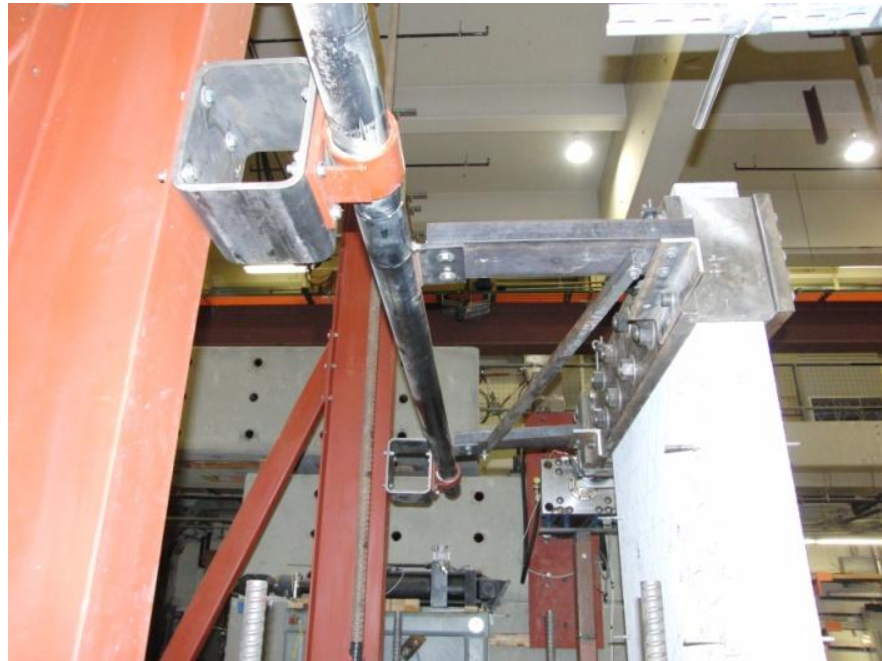
Figure 4-13 Out-of-plane support system
