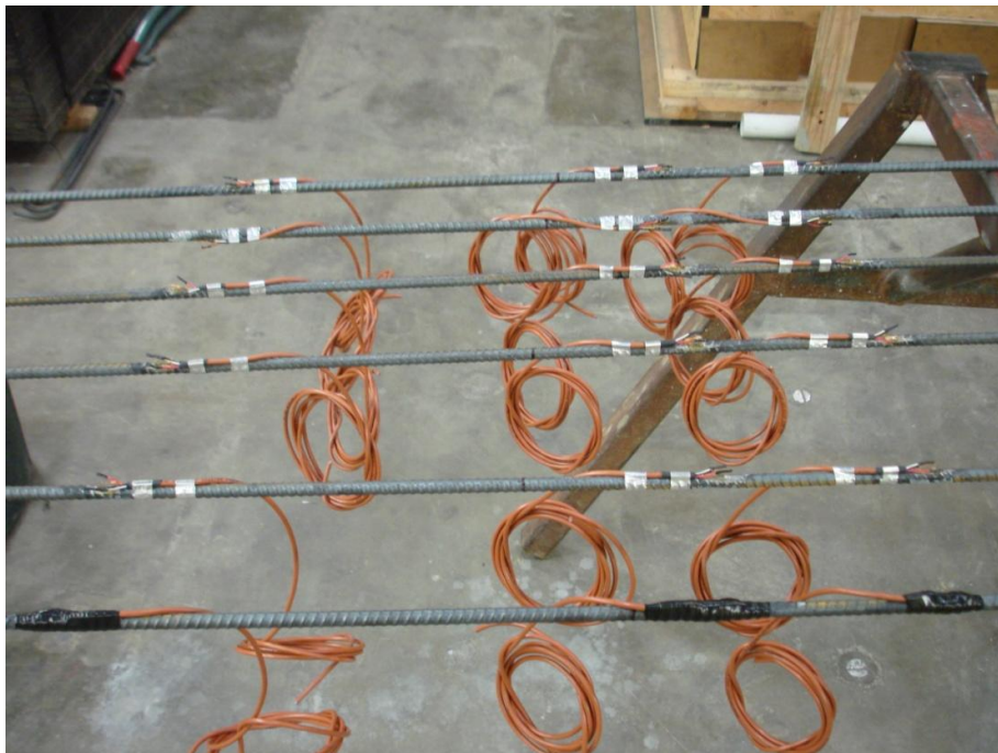
Figure 5-8 Assembling strain gauges on rebars
