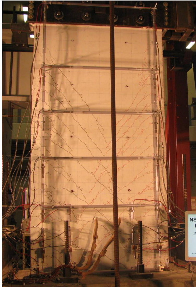
Figure A-3 Crack patterns for RW-A20-P10-S38: (a) 1.1% Drift, and (b) 1.5% Drift
