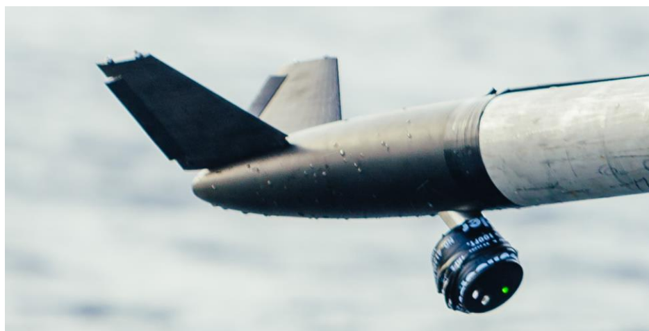
Figure 4 – Control surfaces angled in same direction
