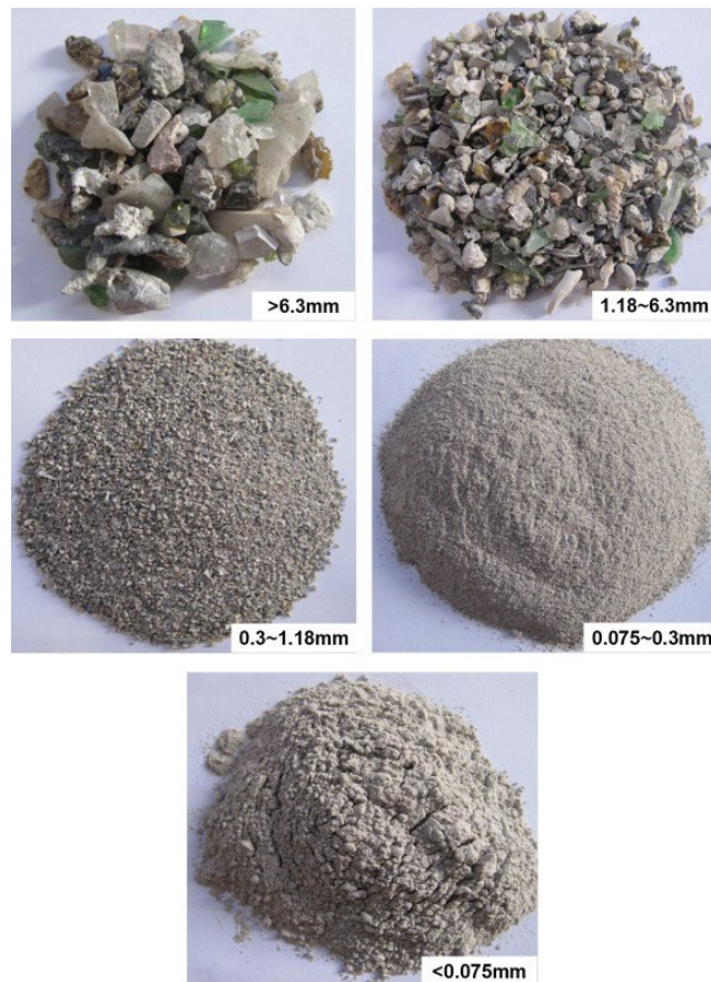
Figure 5.1: Different size fractions of MSW bottom ash used as 20% portland cement replacement in concrete.
