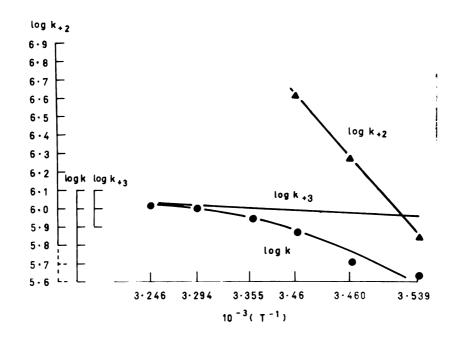
Figure 8: Representation of derived rate constants for acetylation (k ) and de-acetylation (k ) from the Arrhenius plots of eel +2 +3 acetylcholinesterase catalyzed acetylcholine hydrolysis in 100 mM NaCl. Enzyme activity was measured by the pH-stat method with standard assay conditions as indicated in Table XVII. Values of log k were computed from the relationship Vmax = kE. k values were +3 derived from the asymptote of the log k versus reciprocal absolute
