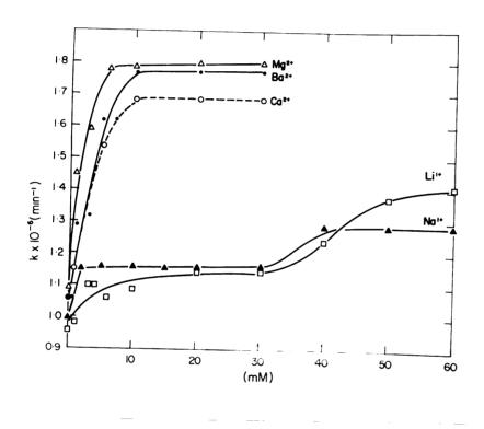
Figure 13: Ionic activation of eel AChE catalyzed acetylcholine hydrolysis. Enzyme activity was measured by the pH-stat method with standard assay conditions as described in the legend of Table XVIII. All ions as indicated were present in the form of chloride salts.
