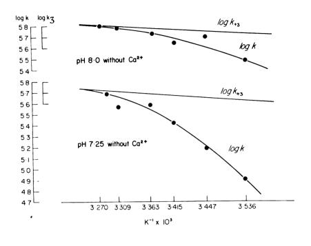
Figure 9: Representation of derived rate constants for acetylation (k) and de-acetylation (k) from the Arrhenius +2 +3 plots of brain acetylcholinesterase (mol. wt. 240000) catalyzed acetylcholine hydrolysis. Enzyme activity was measured by the pH-stat method with standard assay conditions as indicated in Table IV. Values of the rate constants were determined as indicated in Figure 8.
