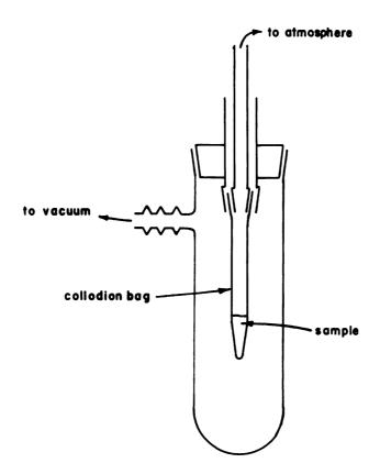
Figure 6: Diagram of the collodion bag vacuum filtration
