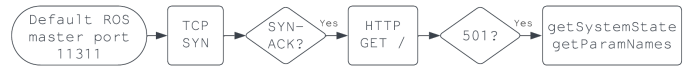
Fig. 1: Overview of ROS 1 scanning procedure. 501 refers to the expected response of error code 501 Not Implemented to HTTP GET / requests sent to the ROS 1 master port [16]. getSystemState and getParamNames are the passive commands (§III-A) used to retrieve information from ROS 1 instances [16].
