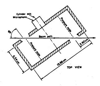
Fig. (1) Cross Section of Windowless Spectrophone
