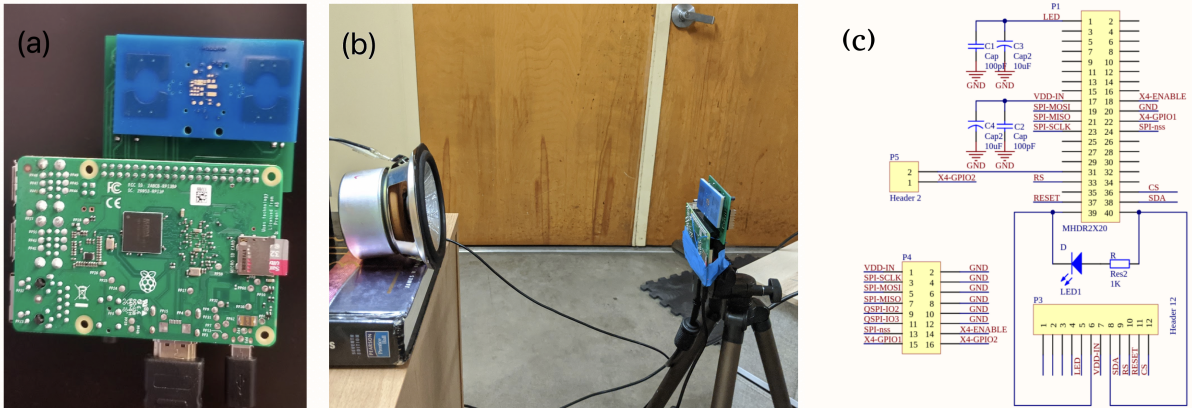
Figure 4.2: Hardware components overview of the UWB audio sensing system: (a) Hardware appearance (b) Proof-of-concept experiment setup (c) Hardware Connection
