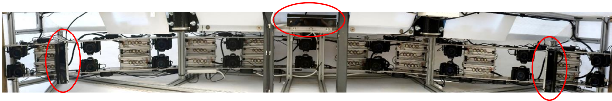
Figure 5. View of the arc mounted on the Spider taken from the ground looking up at the sensor placement (black objects). The Kinects are circled in red.
