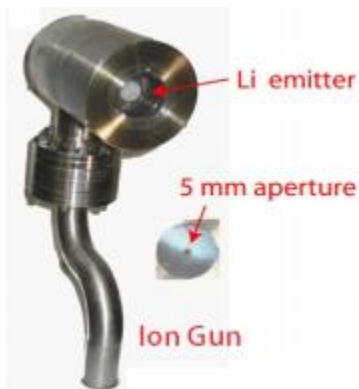
Figure 2.3.2 Picture of the ion gun housing. [11] The Lithium ion source can be seen in the absence of the 5mm aperture. Leads for the heating circuit and biased grids run out through the ion gun shaft.
