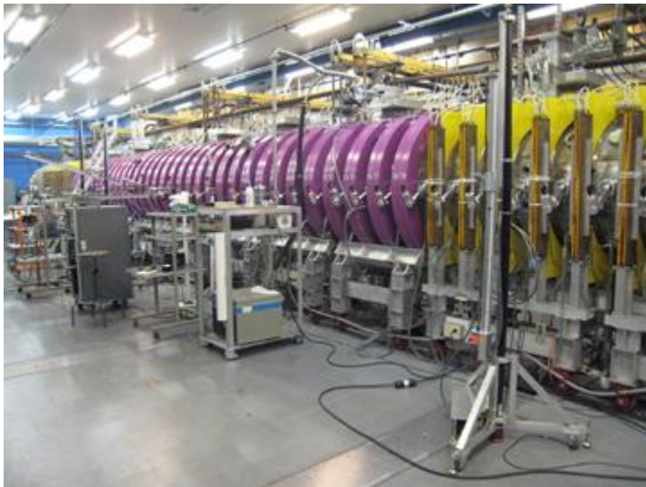
Figure 2.1.2 Picture of the upgraded Large Plasma Device at the BAPS. The purple coils shown are responsible for generating the axial magnetic field. Smaller probes are inserted into flanges attached to circular ports, while larger equipment requires rectangular port access (not shown).
