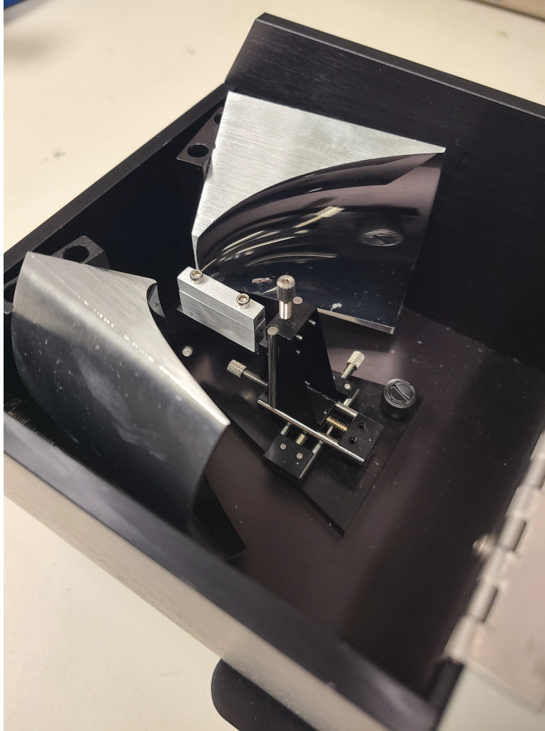
Figure 3.2: Photograph of FTIR sample compartment with beam condenser and polished SW66 sample.
