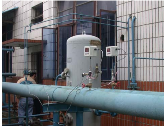
Figure 2 flow measurement with insertion-type mass flow meter
