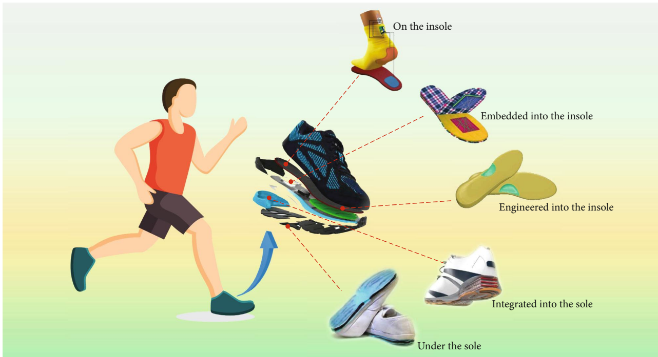
FIGURE 1: Diverse applications of TENG enabled smart shoes for mechanical-to-electrical energy conversion. On the insole. Reproduced with permission from [129]. Copyright Elsevier, 2017. Embedded into the insole. Reproduced with permission from [130]. Copyright Elsevier, 2017. Engineered into the insole. Reproduced with permission from [131]. Copyright Royal Society of Chemistry, 2019. Integrated into the sole. Reproduced with permission from [132]. Copyright Springer Nature, 2015. Under the sole. Reproduced with permission from [133]. Copyright Springer Nature, 2016.
