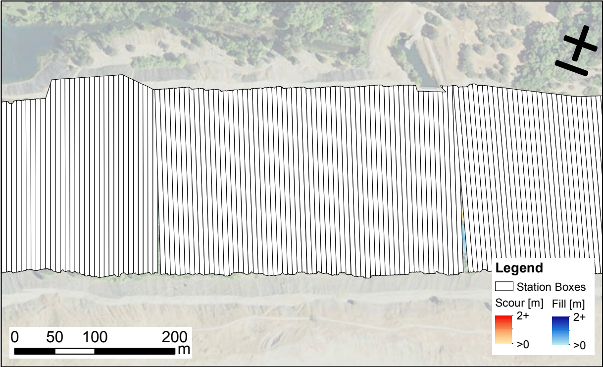
Fig. S9. Station boxes used for creating longitudinal profiles of erosion and deposition volumes and percent area. The boxes are 1.524 m wide (5-ft), orthogonal to the valley centerline, and clipped to the width of the river valley.
