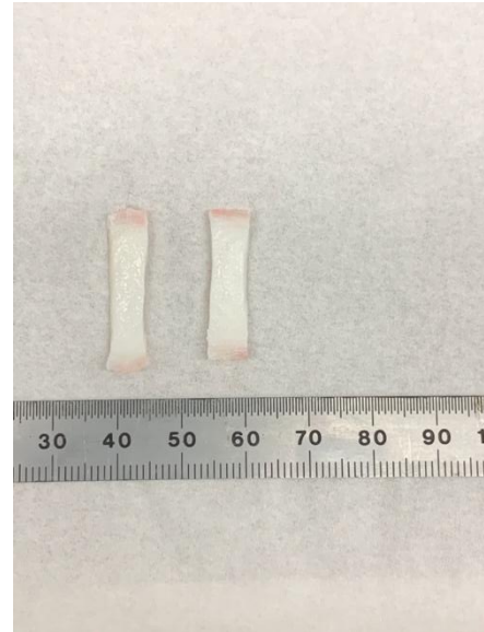
Fig. 4: Prepared tensile specimens (unnotched)
