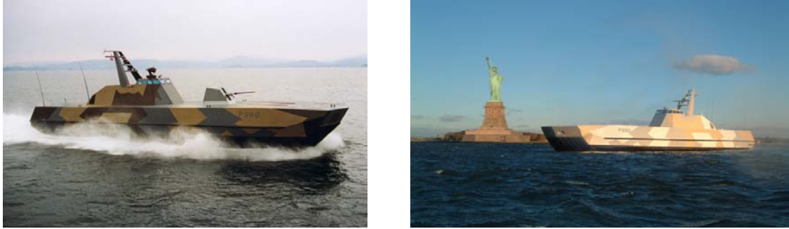
Figure 2-1: Skjold class patrol boat built with FRP sandwich
