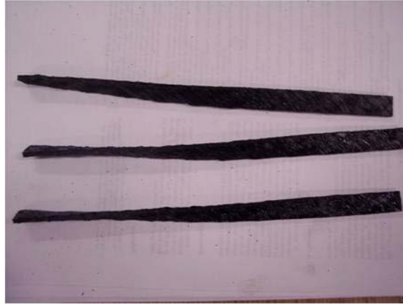
Figure 4-19: Test specimens distorted by asymmetry in process of thermal expansion and contraction after exposure to 260°C for 8 hrs
