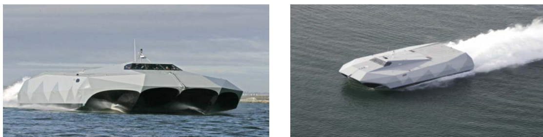
Figure 2-3: M80 Stiletto built with new carbon-fiber materials
