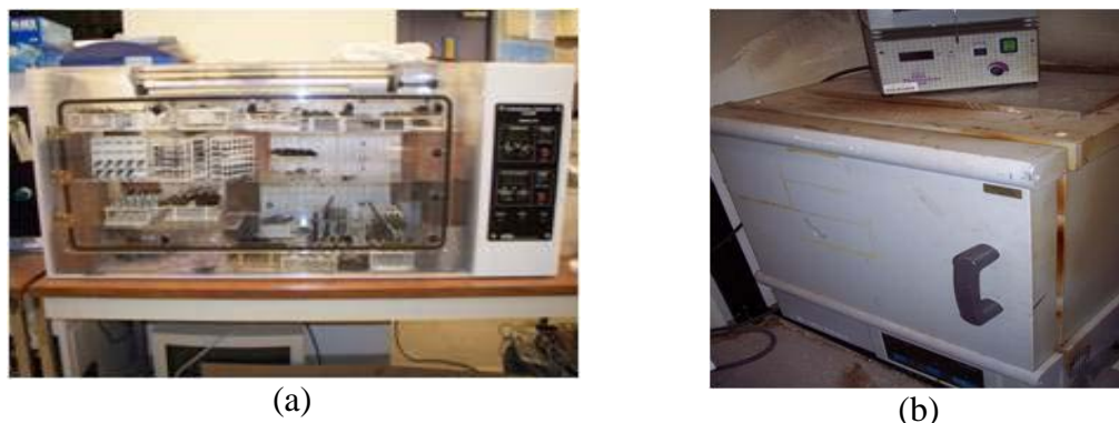
Figure 3-2: (a) Humidity chamber for initial condition and (b) Oven for environmental conditions
