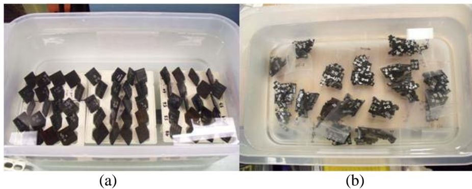
Figure 3-3: (a) Test specimens for water uptake tests and (b) Test specimens for SBS tests immersed in seawater and DI water.
