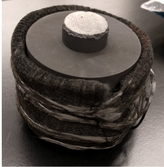
FIGURE C2. Image of the assembly of powders into the SPS graphite die; graphite foil was used between the die and powders. 4YSZ powders were sintered in a Fuji SPS 825-S with parameters of 100°C/minute heating rate, 65 MPa pressure, 1600°C sintering temperature, 10 minute hold time, and 200-300°C cooling rate.
