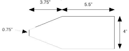
box you plan to use to hold the paddles. The phototubes that we used had a diameter of 3/4". We used the following dimensions for the scintillators:
