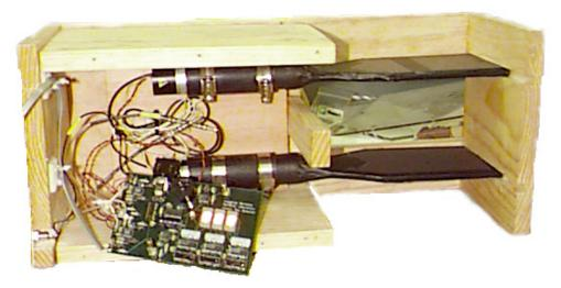
The wood pieces are attached using wood screws and a screwdriver. Afterwards, you should sand and stain the box to protect its surface. The Lucite piece is not attached until after the coincidence circuit has been assembled and attached to it.
