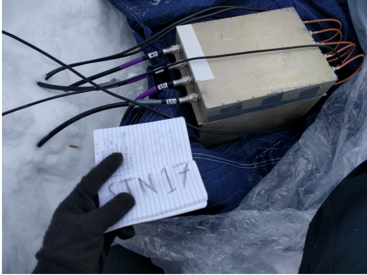
Figure 2.1: Photo of ARIANNA DAQ box as deployed in Moore’s Bay, showing the protective plastic bag and thermal blanket.
