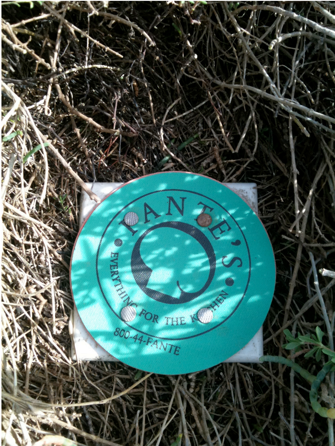
Figure 2: Sediment deposition disk placed in low marsh zone.
