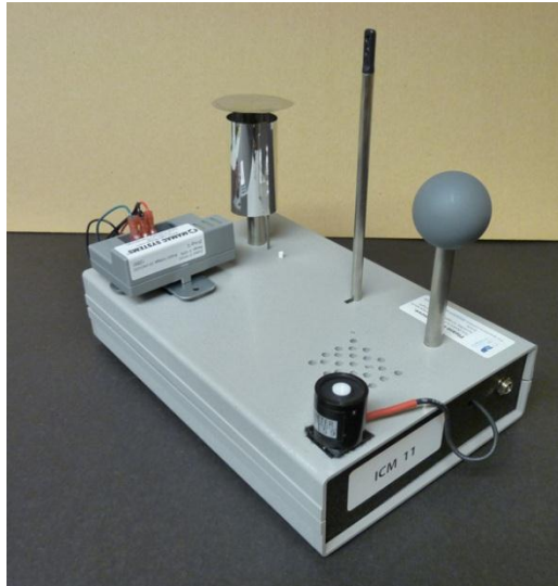
Figure 2: ICM Device With CO 2 , Illuminance, Globe, Air Velocity, Bulb Temperature, and Relative Humidity
