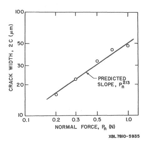
Fig. 3 A plot of the lateral crack width as a function of the normal force  $^3$ , indicating the  $\mathrm{P_n}^{2/3}$  relation.
