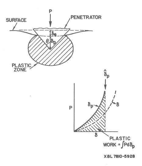
Fig. 6 A schematic indicating the elastic  $\delta_1$  and plastic  $\delta_p$  penetrations by a fixed profile indenter.
