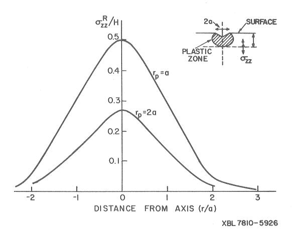
Fig. 1 The spatial dependence of the residual tensile stress along a plane through the intersection of the plastic zone with the penetration axis: the stresses were estimated from an analytic elastic/plastic solution for a spherical cavity and an elastic solution for a half space.
