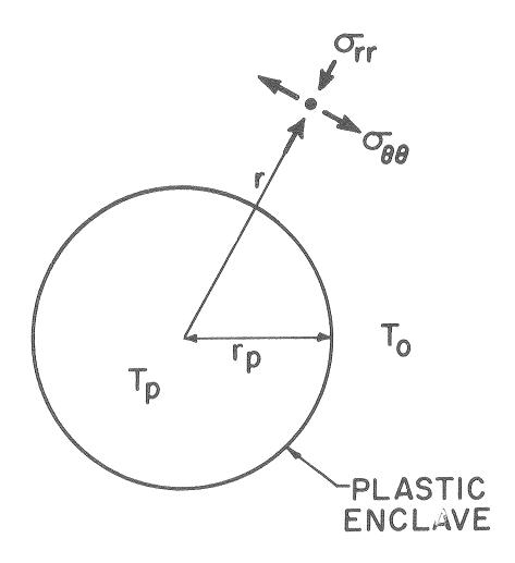
Fig. 7 A plastic enclave in an elastic matrix indicating the stresses developed by heat genration in the plastic zone.
