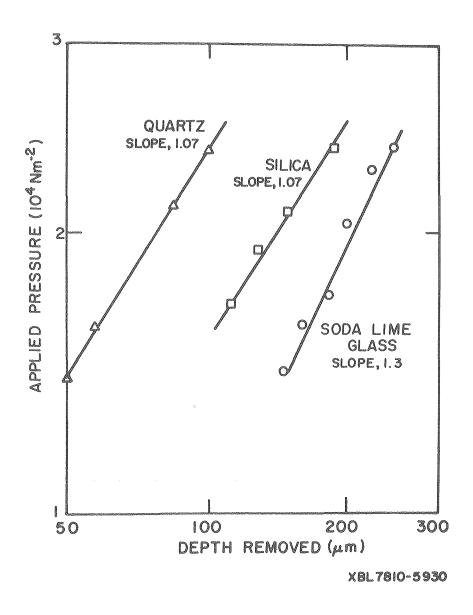
Fig. 4 A plot of the material removed as a function of the applied force  $^{15}$ .
