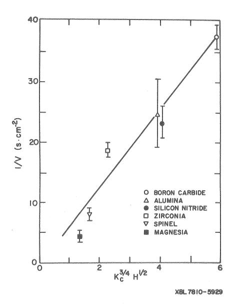
Fig. 5 A plot of the inverse of the material removal against the material dependent parameter  $\rm K_{\rm C}^{2/3}~H^{1/2}~predicted$  by the lateral fracture analysis.
