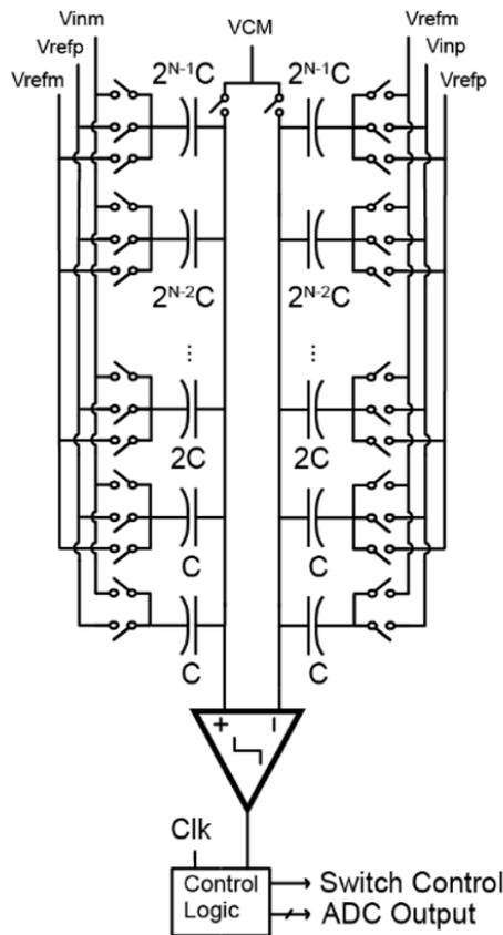
**Figure 3.30:** Schematic of EMCS SAR ADC on FM-ExG gateway integrated circuit.
