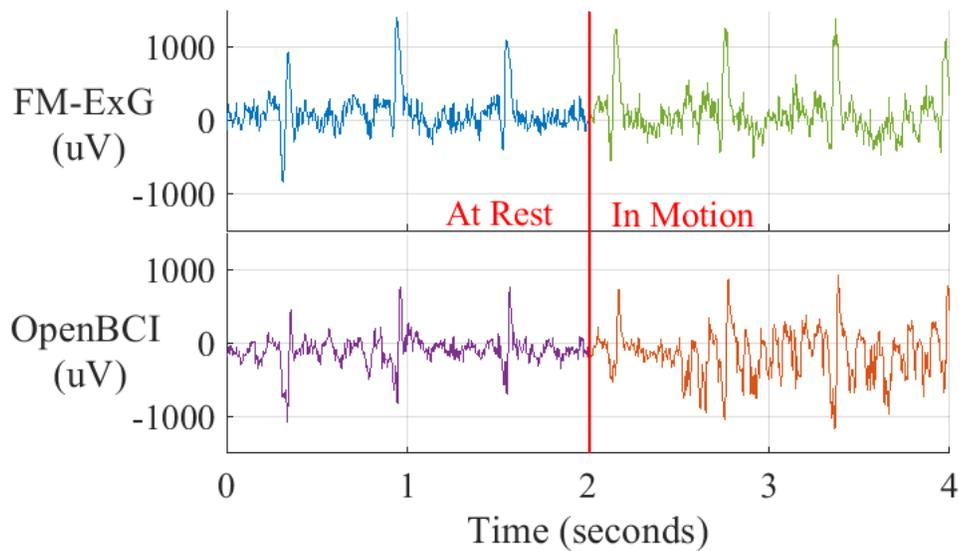
**Figure 3.20:** Comparison between FM-ExG and OpenBCI transient traces during subject motion.
