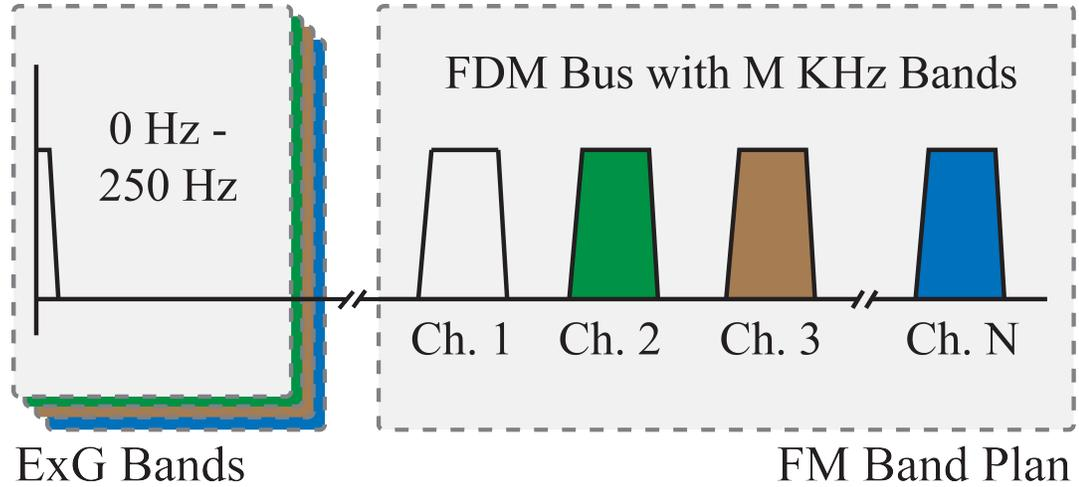
**Figure 3.4:** Frequency domain representation of ExG message signals and their mapping to the system's FM-FDM bus.
