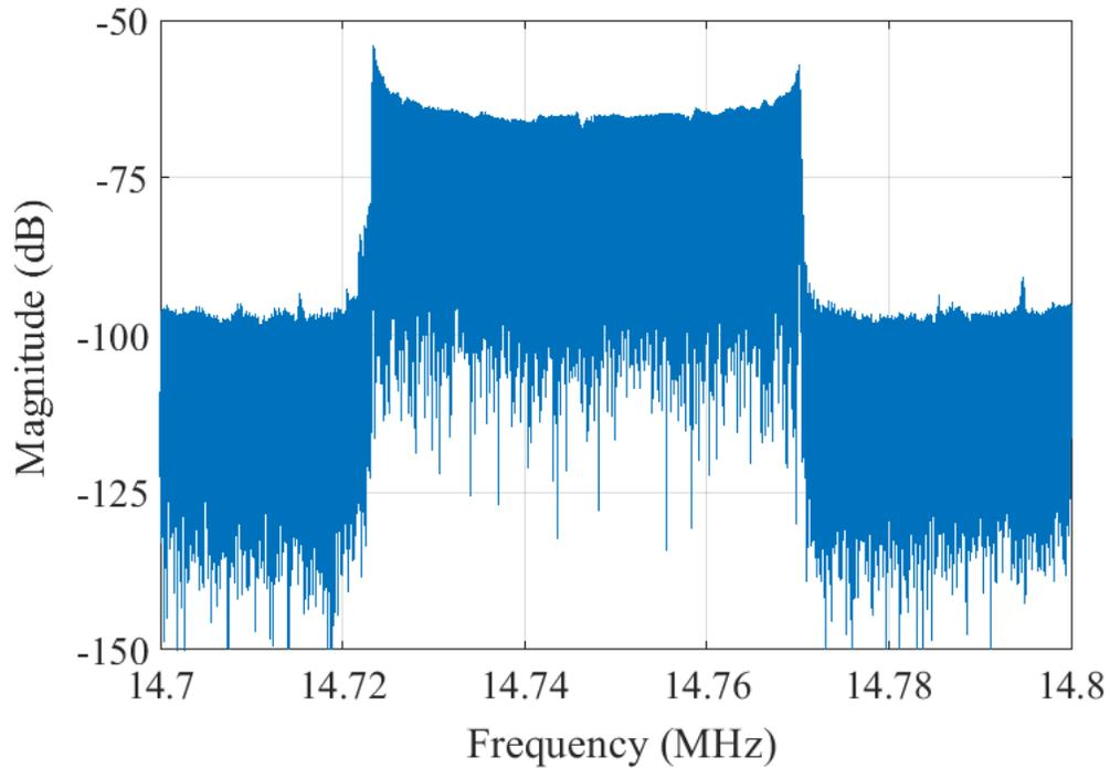
**Figure 3.10:** A single active electrode’s FM output in the frequency domain.
