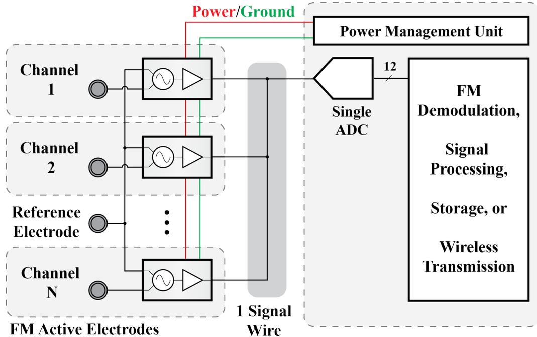
**Figure 3.2:** Block diagram of distributed FM-ADC biopotential recording system.
