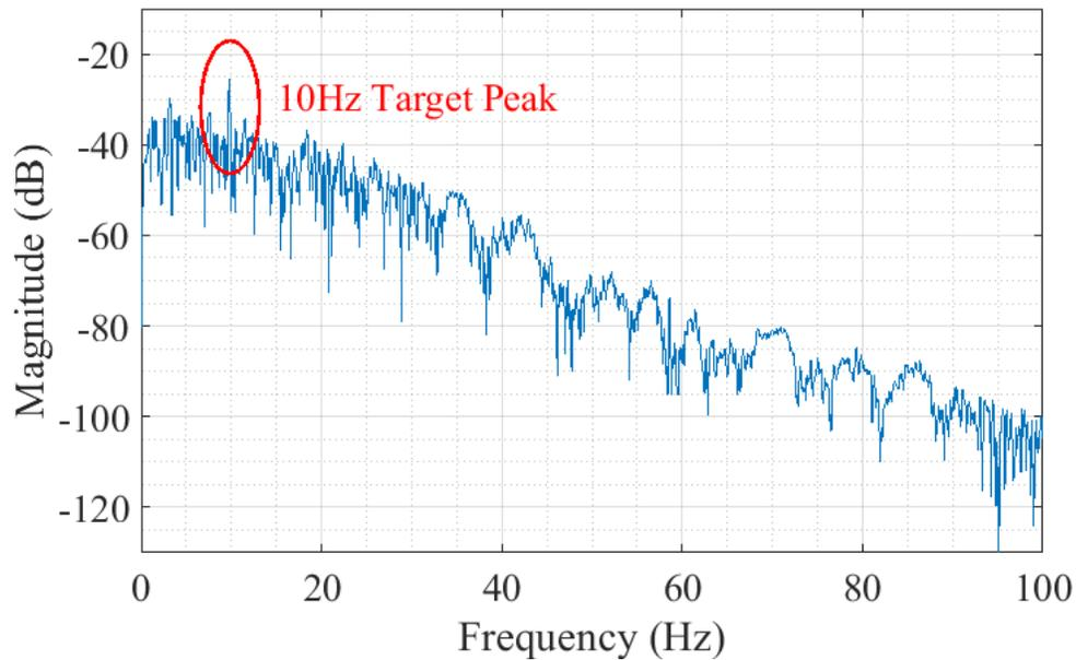
**Figure 3.24:** Frequency components in FM-ExG recording during SSVEP EEG experiment with 10Hz flashing target.
