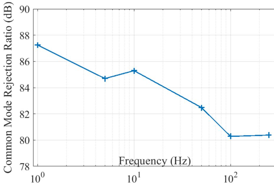
**Figure 3.19:** Active Electrode IC common mode rejection ratio measurements.
