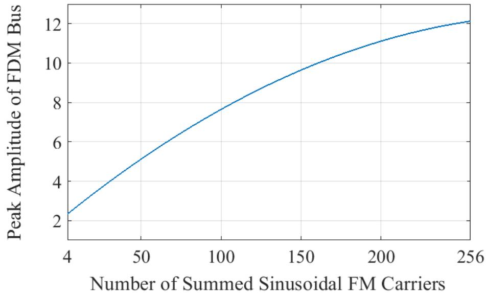
**Figure 3.5:** MATLAB simulation results of the three-sigma peak amplitude of summed sinusoidal FM carrier waves.
