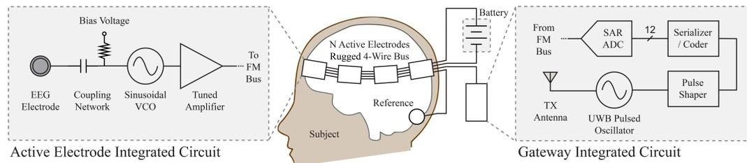
**Figure 3.3:** Block diagram of the implemented robust biopotential recording system using distributed multi-channel FM-ADC and offloaded demodulation.
