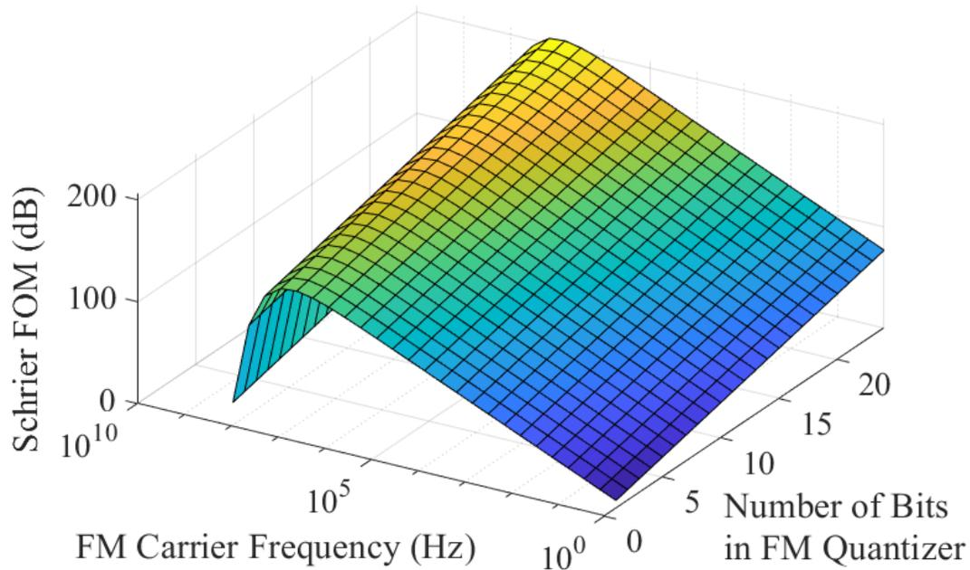
**Figure 4.1:** FM-ADC system Schreier FOM versus FM carrier frequency and number of bits in FM quantizer.
