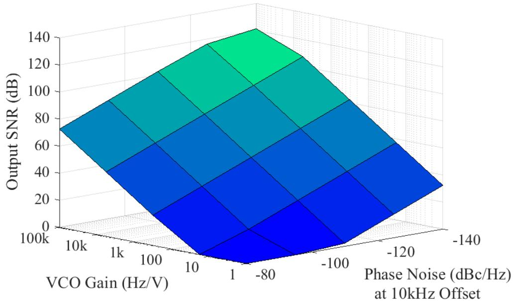
**Figure 3.6:** MATLAB simulation results demonstrating the effect of VCO gain and phase noise on system SNR.
