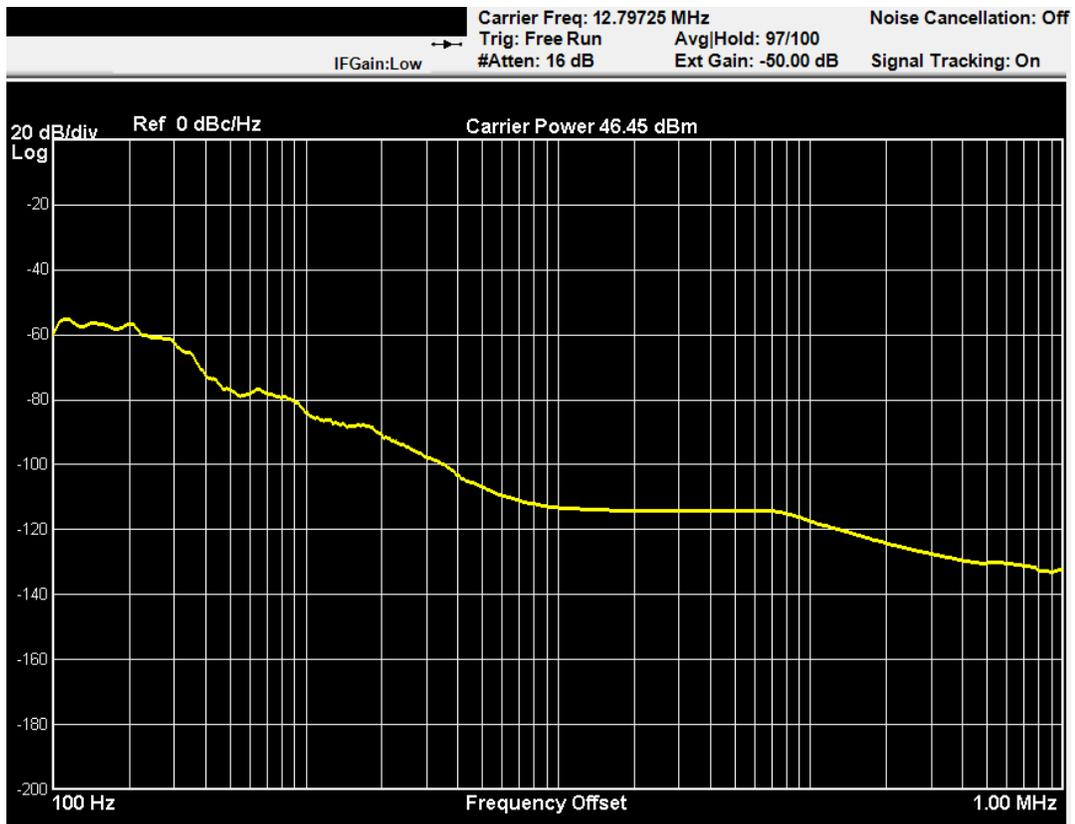
**Figure 3.13:** Measured phase noise of VCO employed for FM modulation.
