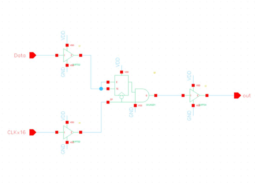
**Figure 3.27:** OOK coder schematic diagram from FM-ExG gateway integrated circuit.
