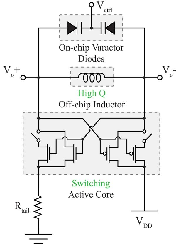
**Figure 3.7:** The voltage-controlled oscillator implemented on the active electrode integrated circuit.
