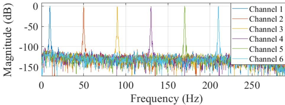
**Figure 3.16:** Demodulated system output in 6-channel test measurement.
