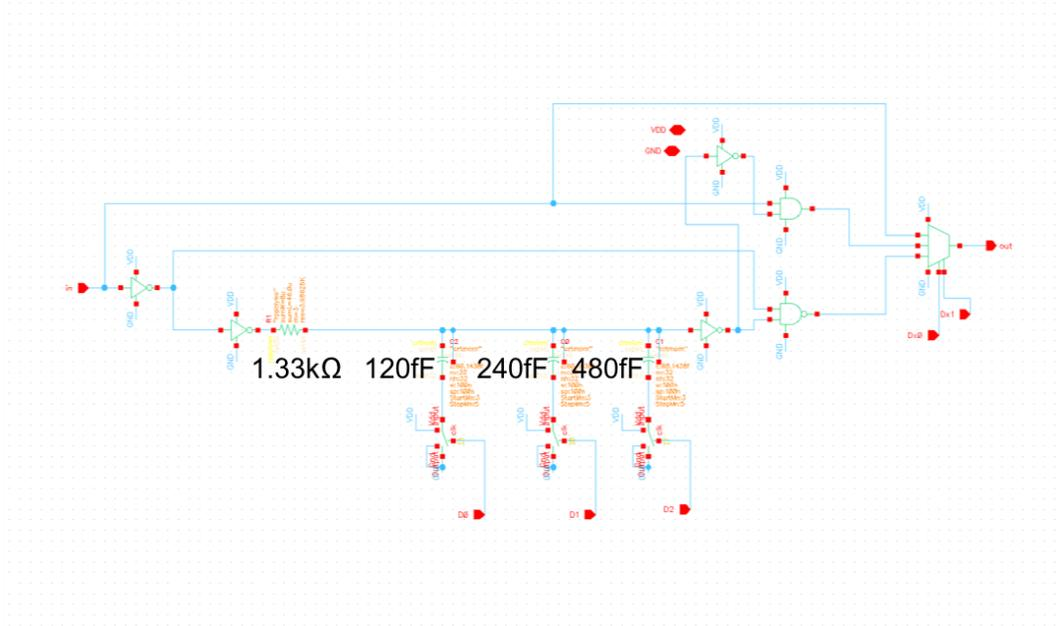
**Figure 3.28:** Pulse shaper circuit implementation diagram from FM-ExG gateway integrated circuit.
