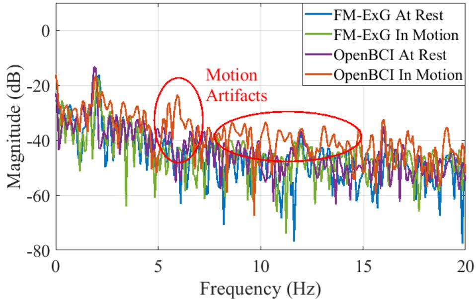
**Figure 3.21:** Comparison between frequency components in FM-ExG and OpenBCI recordings during subject motion.
