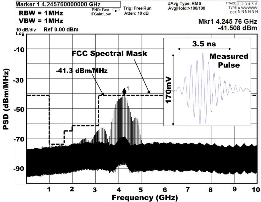
**Figure 3.31:** Measured FM-ExG Gateway IC UWB PSD showing FCC mask compliance and time domain pulse (inset).
