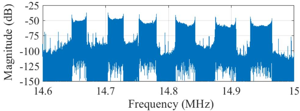
**Figure 3.15:** Frequency spectrum of FM-FDM bus with 6 channels.
