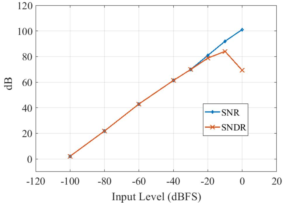
**Figure 3.12:** Measured SNR and SNDR across input voltage dynamic range.
