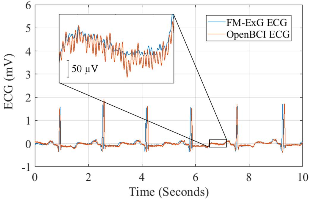
**Figure 3.22:** Comparison between FM-ExG and OpenBCI transient traces with 60Hz power line interference present.
