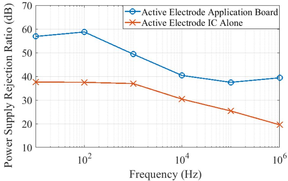
**Figure 3.18:** Active Electrode IC and application PCB power supply rejection ratio measurements.
