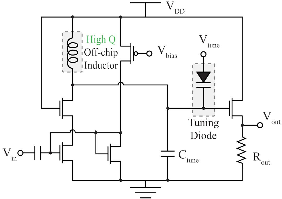
**Figure 3.8:** The bandpass tuned amplifier implemented on the active electrode integrated circuit.
