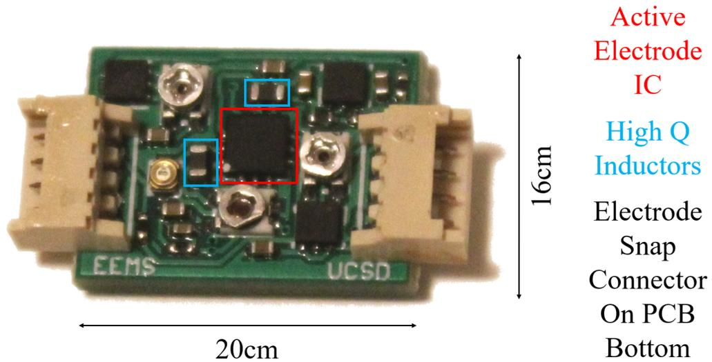
**Figure 3.17:** Active Electrode IC application printed circuit board.
