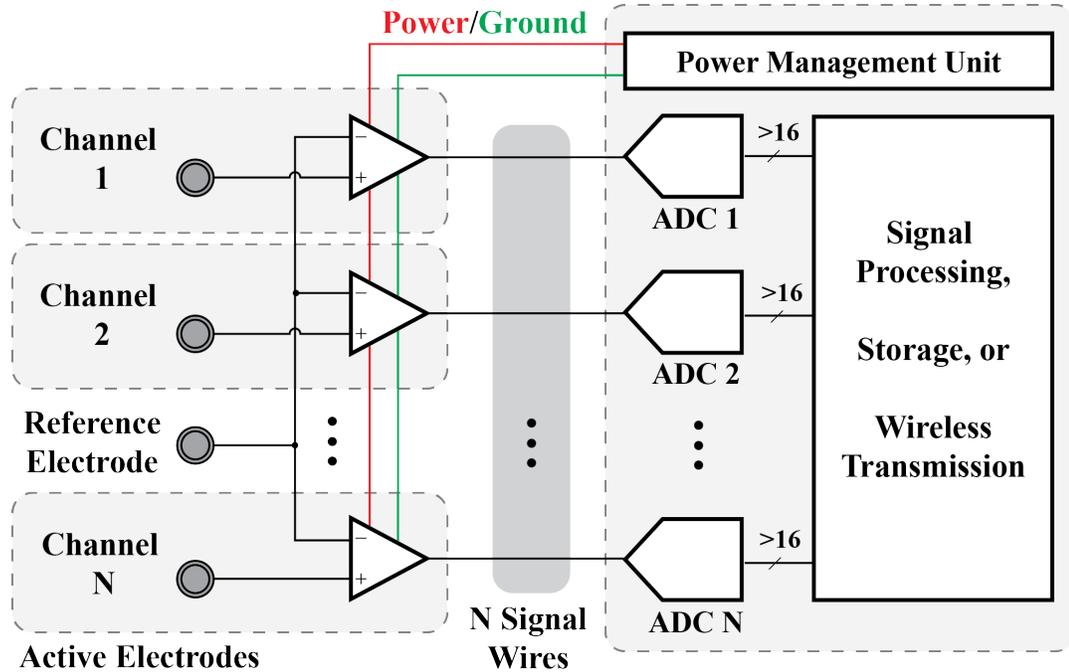
**Figure 3.1:** Block diagram of traditional N-channel biopotential recording system.
