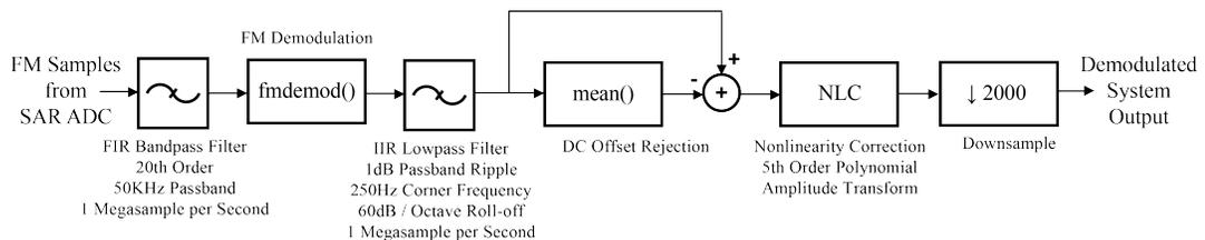
**Figure 3.9:** The demodulation scheme implemented in MATLAB that was used for all analog performance measurements.
