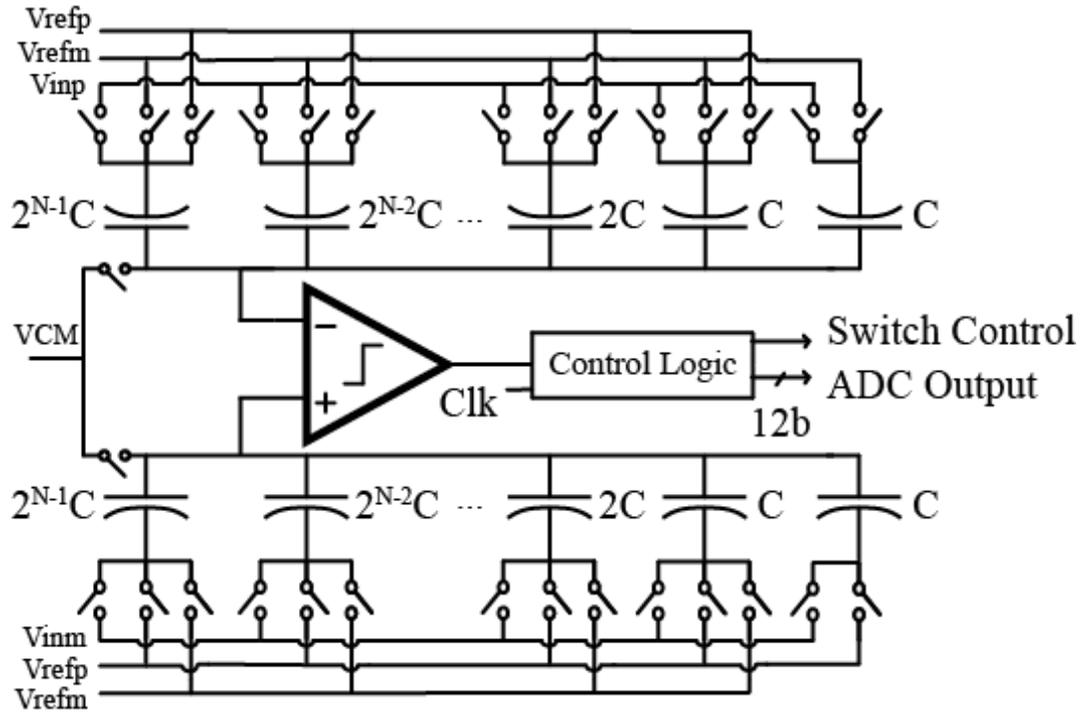
**Figure 2.4:** FM-ADC internal SAR ADC diagram.
