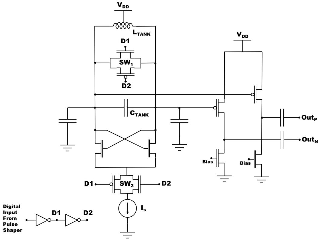
**Figure 3.29:** Schematic of pulse generator for IR-UWB transmitter on FM-ExG gateway integrated circuit.
