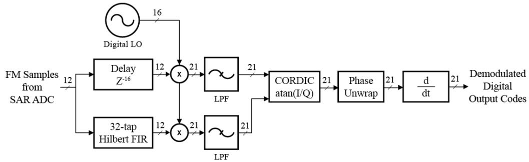
**Figure 2.5:** FM-ADC demodulation digital signal processing block diagram.
