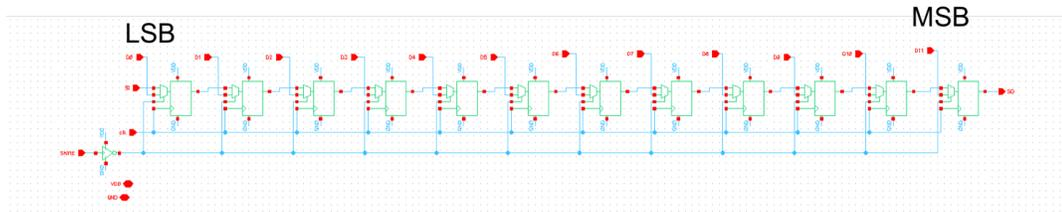
**Figure 3.26:** Circuit schematic of shift register based PISO used to serialize the output of the FM-ExG gateway SAR ADC prior to coding for UWB.
