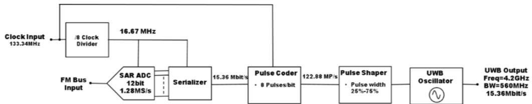
**Figure 3.25:** Top level block diagram of FM-ExG gateway integrated circuit.
