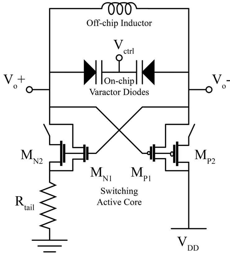
**Figure 2.3:** Current reuse voltage-controlled oscillator.
