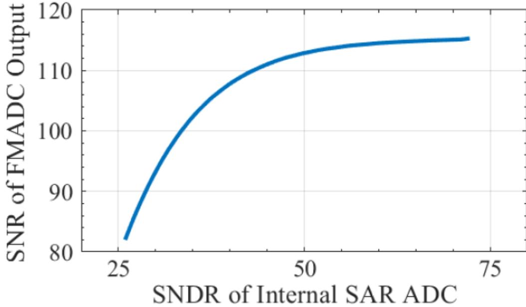
**Figure 2.7:** Simulated effect of SAR SNDR on FM-ADC output SNDR.
