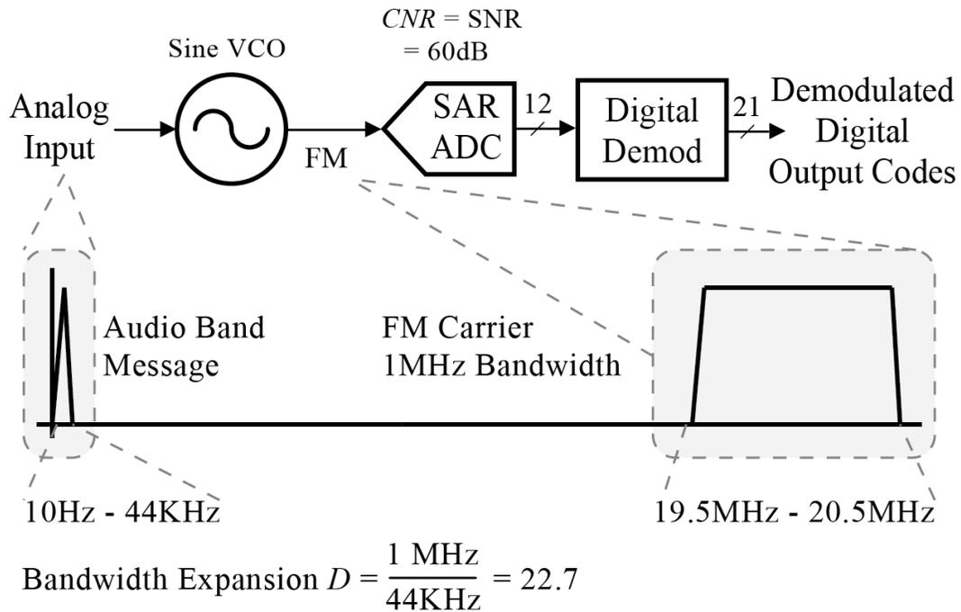
**Figure 2.1:** Block diagram of proposed FM-ADC.
