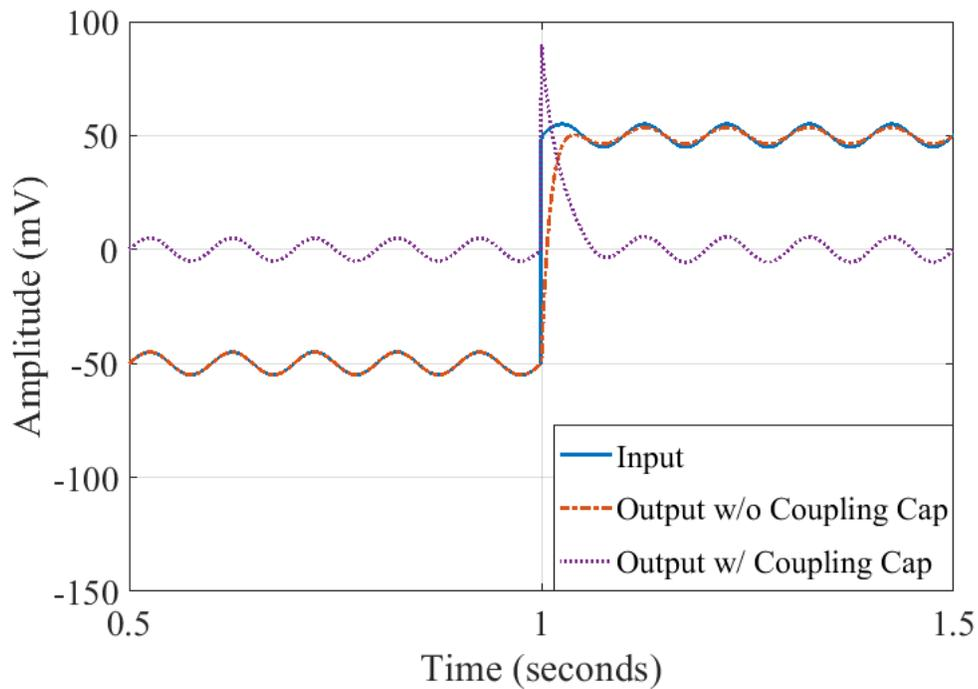
**Figure 3.14:** Demodulated system output for 100mV step voltage at active electrode input.
