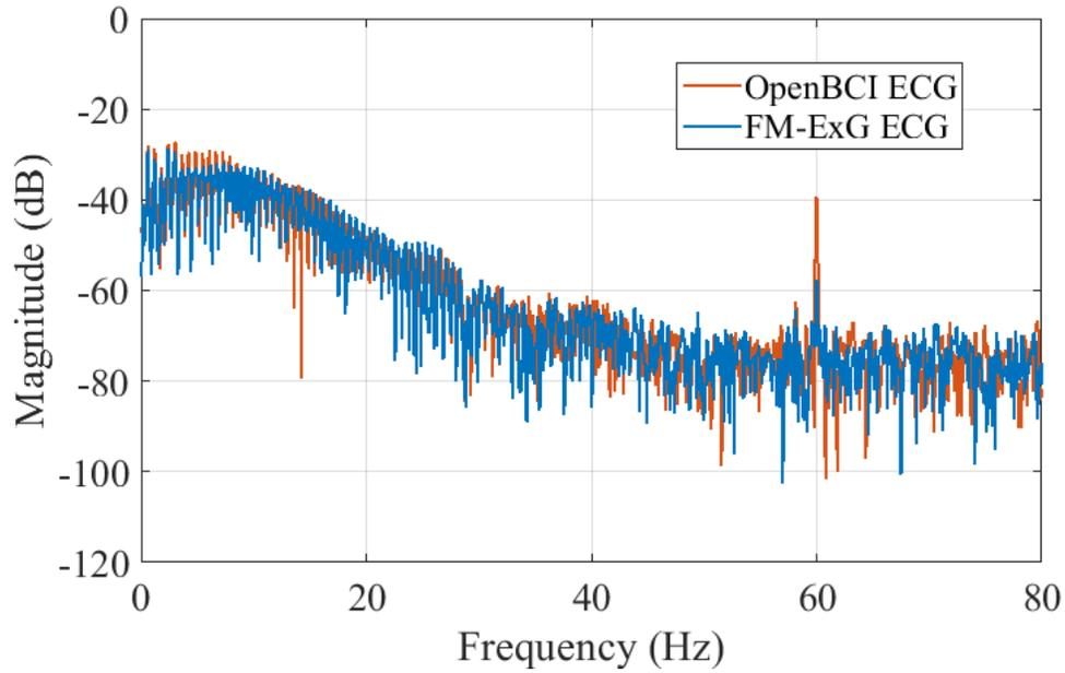
**Figure 3.23:** Comparison between frequency components in FM-ExG and OpenBCI recordings with 60Hz power line interference present.
