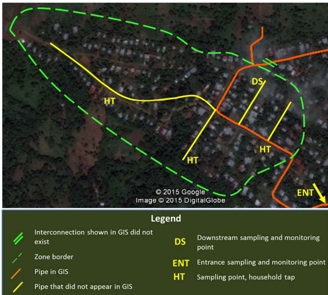
Figure 2.5: Schematic of Zone 3. The point where pressure and entrance flow were measured (ENT), was located outside the image, approximately 1 km to the southeast of the bottom right corner of the diagram. The pump station discharge (PD) where water quality grab samples were collected and continuous pressure, chlorine and turbidity monitoring took place, was located approximately 400 m to the south (upstream) of ENT.
