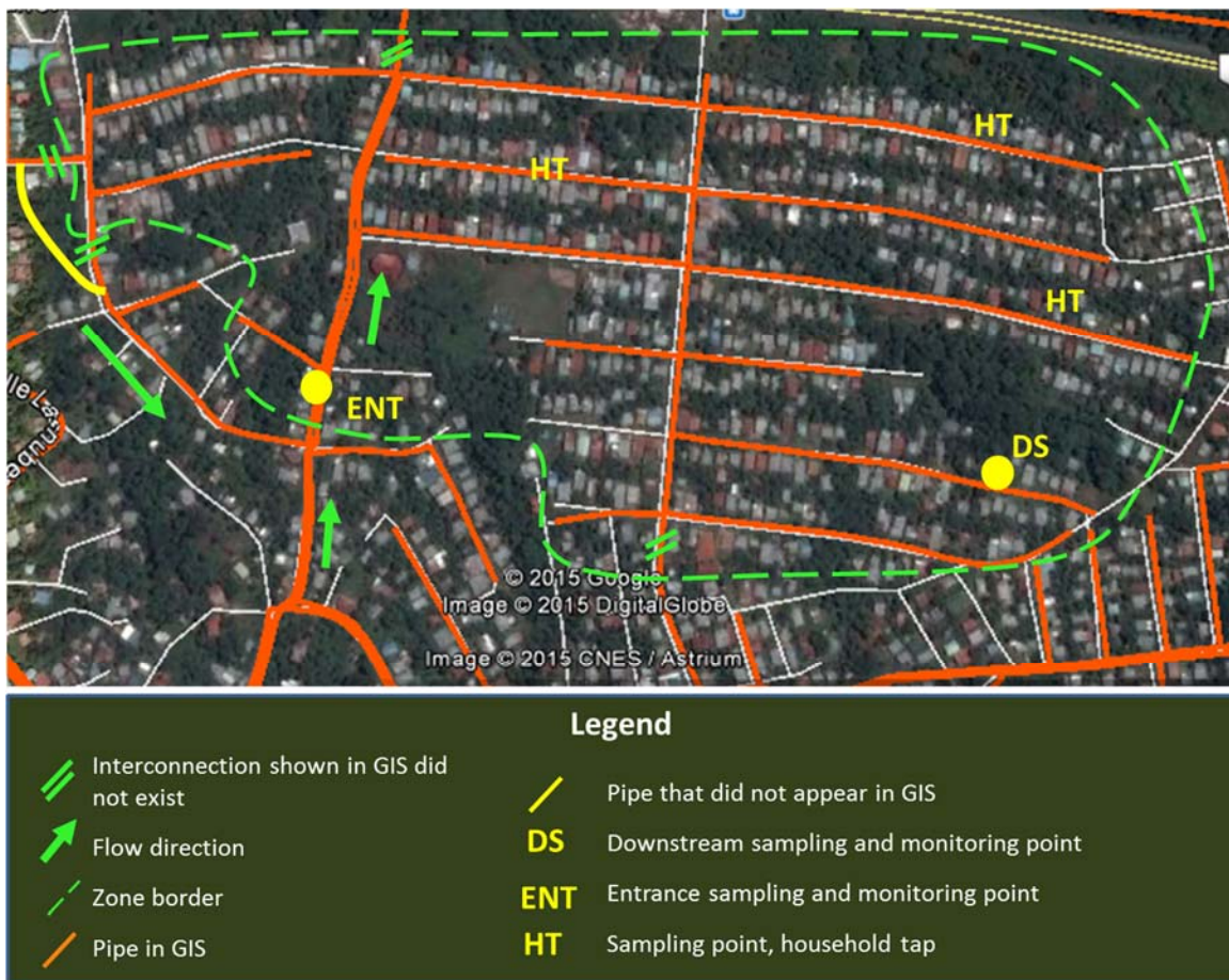
Figure 2.4: Schematic of Zone 2. Some differences between the network's configuration in IDAAN's GIS database and its actual configuration were found during field inspections to verify the isolation of this zone.
