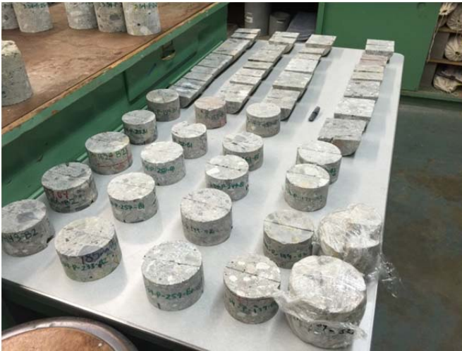
Figure 2.9: Concrete cores for visual inspection.
