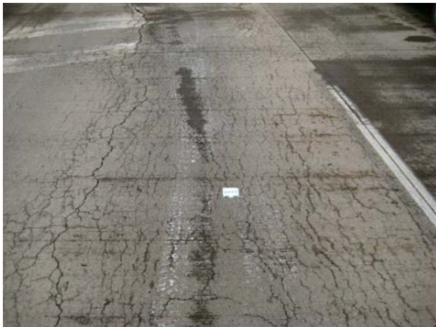
Figure A.2: Example photos showing some of the common petrographic features of ASR ( cont'd ).
