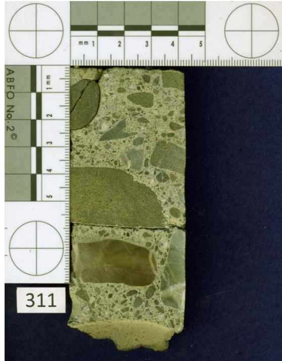
Figure 3.4: Example scans of the cut surfaces of three bridge cores.
