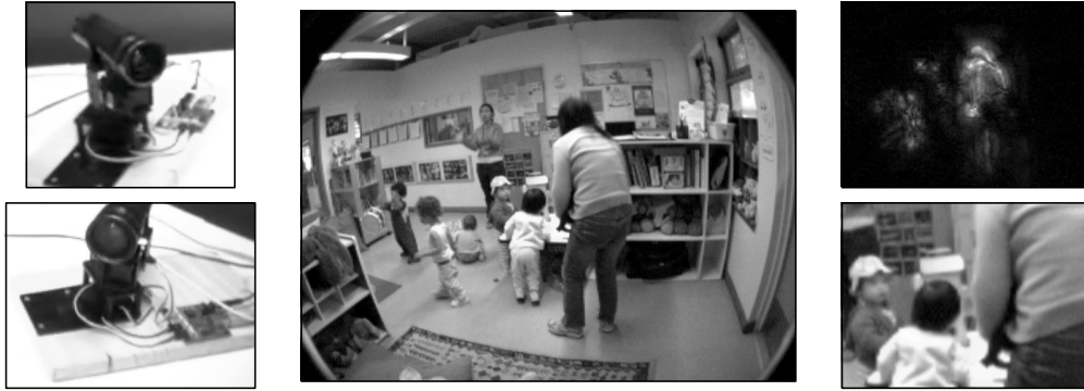
Figure IV.7 A simple robotic camera (left) collected 160^\circ images at 640 \times 480 resolution (center) and compute saliency maps (top right). The camera then orient towards the most salient pixel. After movement, a snapshot is taken (bottom right).
