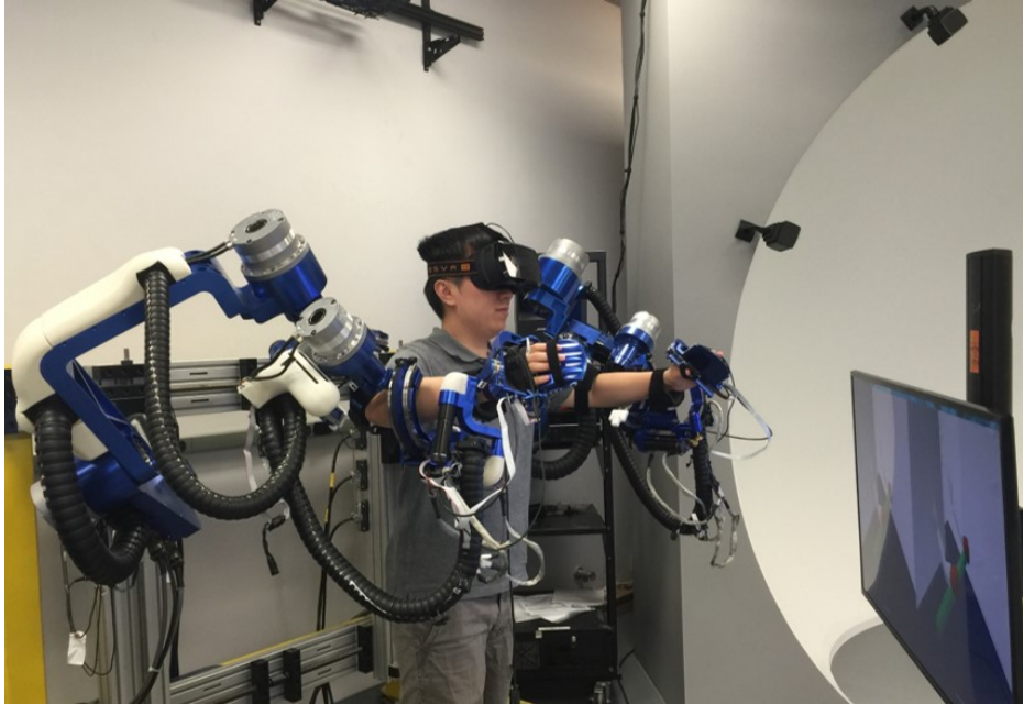
Figure 6.5: A subject is interacting with virtual reality “Reach” game via the wearable exoskeleton.
