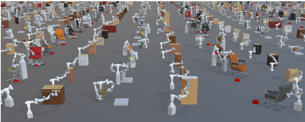
Figure 1.1. A subset of environments in ManiSkill. We currently support 4 different manipulation tasks: OpenCabinetDoor, OpenCabinetDrawer, PushChair, and MoveBucket; each features a large variety of 3D articulated objects to encourage generalizable physical manipulation skill learning.
