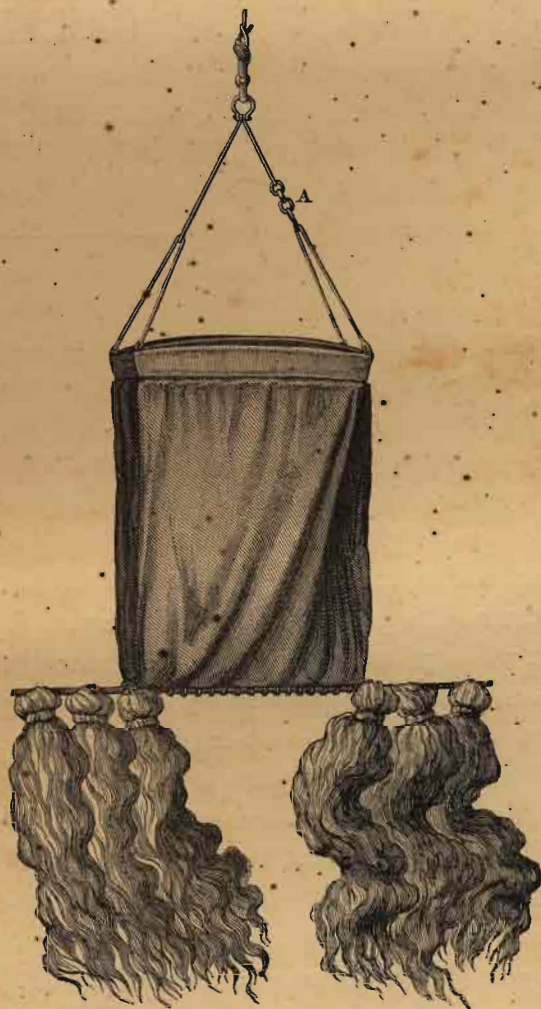
FIG. 2.—Dredge with "hempen tangles."
