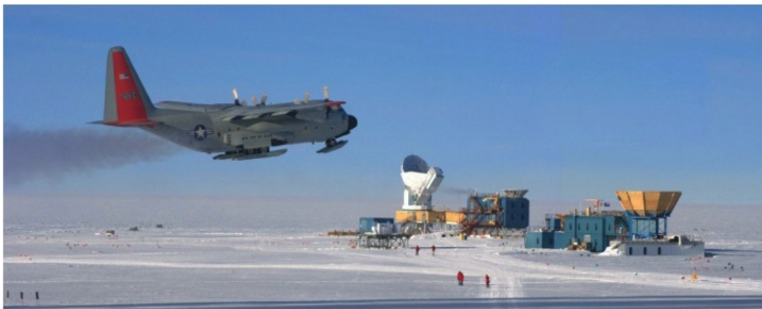
Figure 4.2: The Dark Sector of the Amundsen-Scott South Pole station, where the CMB experiments are located. In the foreground is an LC-130 cargo plane used to transport personnel, food, fuel, scientific equipment, etc. to and from the station. LC-130s are outfitted with skis (visible just below the plane) to enable them to land on the snow-pack at the pole. In the center of the picture stands the South Pole Telescope, with the building which housed BICEP1 and BICEP2 directly to the right. To the right of these is the Martin A. Pomerantz observatory (MAPO) which currently houses the Keck array. The small red dots towards the bottom of the picture are researchers walking towards the Dark Sector wearing the “Big Red” extreme cold weather (ECW) jacket.
