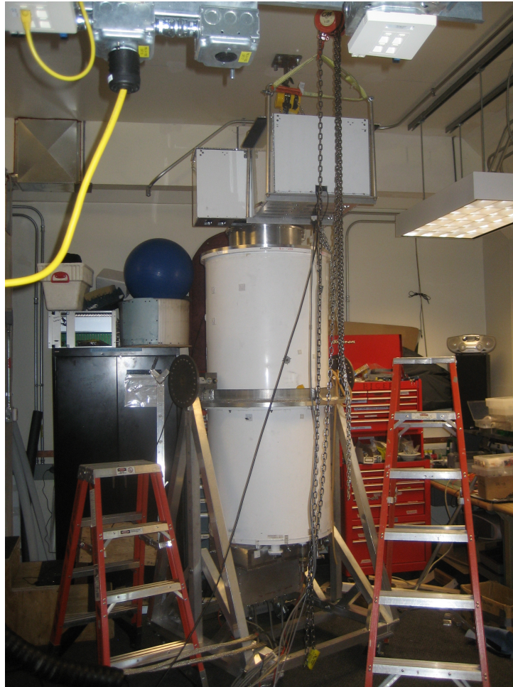
Figure A.2: The FTS coupled directly to the BICEP2 cryostat prior to decommissioning at the South Pole in December 2012. The mount is just off screen to the left.
