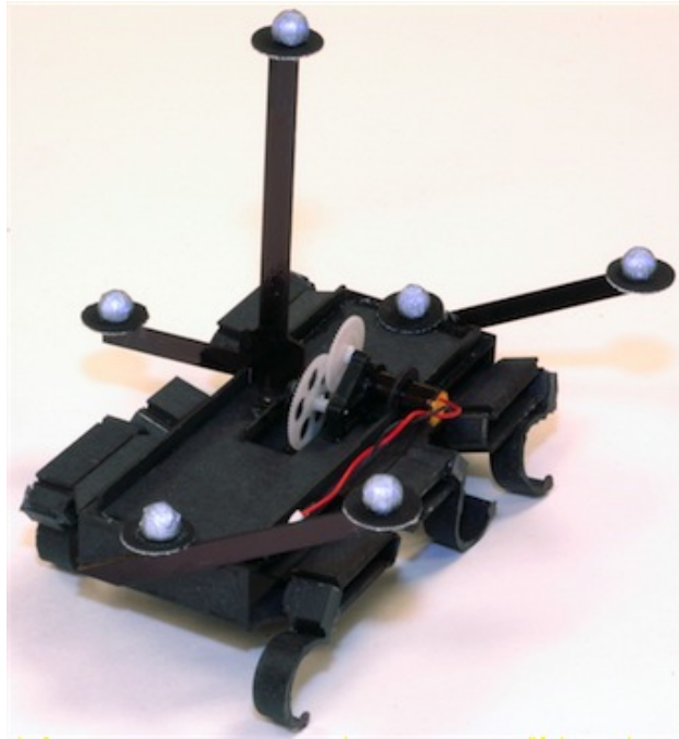
Figure 5.8: The robot chassis with rigid tracking geometry and retro-reflective spheres attached.
