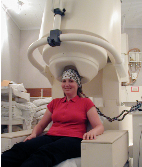
Figure 1.2 Shown above is the MEG system (VSM MedTech, Coquitlam, BC, Canada) installed at the UCSF Biomagnetic Imaging Laboratory. The helmet above the volunteer contains the SQUID-based magnetic field sensors, while the large cylindrical dewar contains liquid helium to cool them to their superconducting operation temperature. The subject is shown wearing a high-density electrode cap for optional simultaneous recording of EEG.
