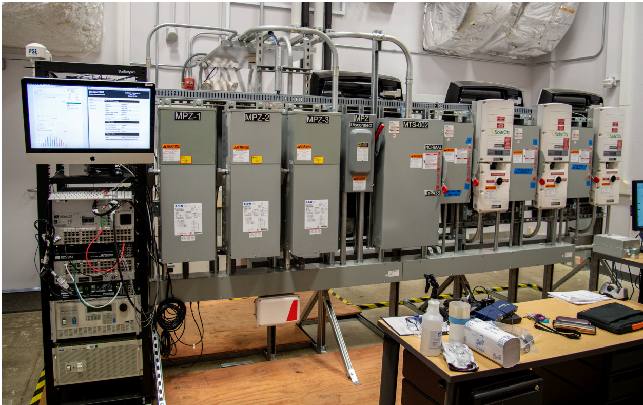
Figure 21: FLEXGRID HIL testing setup. © 2010-2019 The Regents of the University of California, Lawrence Berkeley National Laboratory. Photo Credit: Thor Swift.
