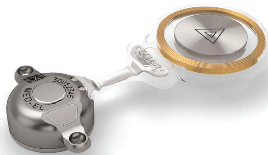
Figure 1. The Bonebridge (MED-EL): the first active transcutaneous bone conduction implant. Provided courtesy of and with permission from MED-EL.
