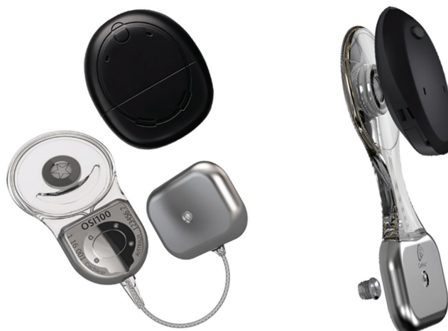
Figure 2. The Osia bone conduction implant (Cochlear) combines an implanted receiver coil and piezoelectric-based actuator, which is anchored to the bone through an osseointegrated implant. Generation 1 (panel 1). Generation 2 (panel 2) with an improved form factor. Illustration provided courtesy of and with permission from Cochlear.
