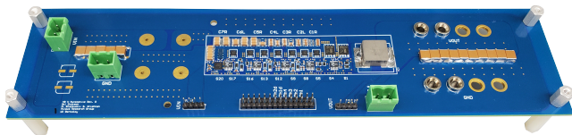
Fig. 1: Photograph of a 48 V to 6 V interleaved-input single-inductor Dickson converter built for demonstration of circuit operation as well EMI mitigation techniques.
