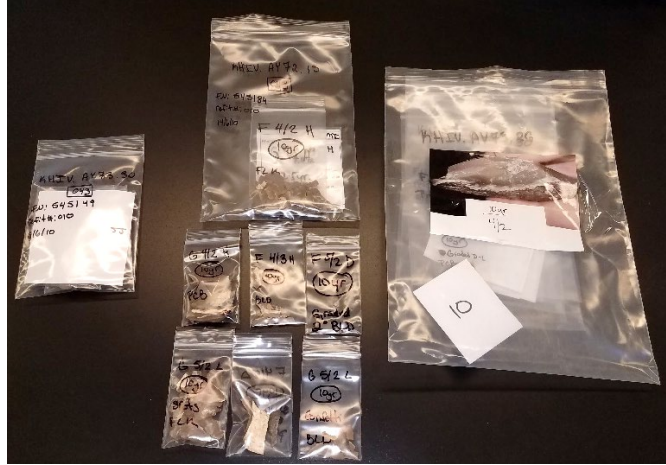
Figure 5.2: This image depicts an RMU that was constructed based on the RMU characteristics listed above. The outer bag is labeled with a photo of the core used to construct the RMU and Munsell color for quick identification.
