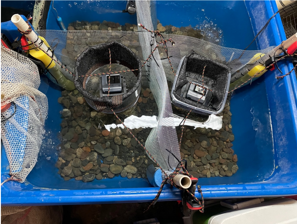
Figure 3.2. Santa ana sucker feeding trial experimental arena set up. The 200-gallon holding tank was separated into four arenas using stainless steel hardware clothe. The bottom of the tank was covered in a shallow layer of river stone. Sharp edges were covered using foam pool noodles to prevent sucker from harming themselves. Powerheads provided flow and aeration. GoPros are depicted in the clear containers used to film the feeding trials.
