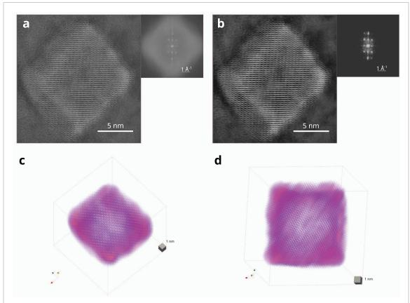
**Figure 2.** Exemplary ptychographic reconstruction (a) before and (b) after denoising. (c) Reconstructed volume, oriented along the [112] direction. (d) reconstructed volume viewed along the [228] direction.
