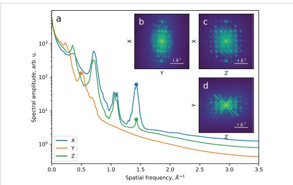
**Figure 5.** The spectral amplitude of the reconstructed volume, projected (via integration) onto axes X, Y, Z (a) and onto planes XY, XZ, YZ (b), (c), (d) respectively). Axes X and Z are perpendicular to the missing wedge, and Y aligns with the missing wedge direction. Points indicate the highest-resolution peak in the power spectrum. Scale bar in (b)–(d)  $1 \text{ Å}^{-1}$ .
