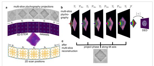
**Figure 1.** Atomic resolution MSPT. (a) Scheme of the reconstruction algorithm and tilt-series 4D-STEM measurements. (b) schematic of the slicing of the volume along the depth direction (*c*) example image of a projected phase image after reconstruction.
