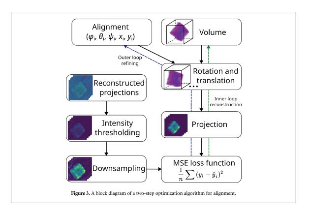
accurately describes the outline of the nanocube. The projection images derived from this mask volume are then applied to the original ptychographic images to mask out substrate contrast outside of the nanocube. This approach compels a subsequent full-scale reconstruction to focus more intensively on the inner structure of the nanocube.
