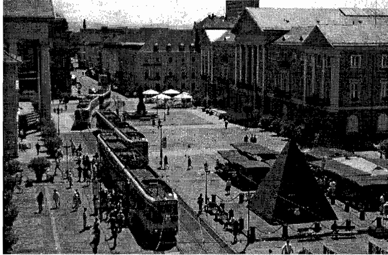
Photo 6.1. Dual-Voltage S-Trains in the Core of Karlsruhe. S-Trains queue for customers at Marktplatz in the heart of the city. The center section of the bi-directional articulated vehicles accommodate the dual-voltage electrical hardware. Speeding up S-Trains within the city limits is a system of induction loops imbedded in surface streets that allow signal preemption. S-Trains are permitted to travel as fast as 50 km per hour while in the city.
