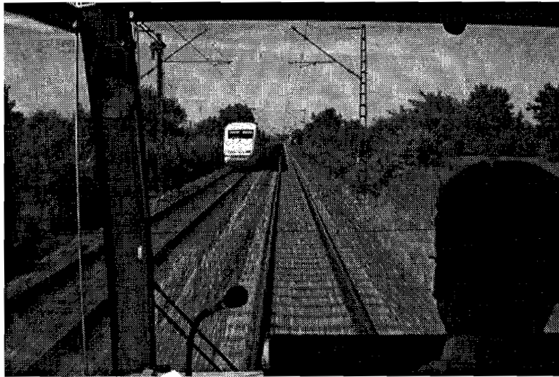
Photo 6.3. S-Train Shares Tracks with a High-Speed Inter-City Train. A view of an on-coming DB high-speed train headed to Switzerland from inside an S-Train. S-Trains operate up to 100 km per hour while sharing DB tracks, faster than the 75 km per hour they travel while on separate tracks in the suburbs.
