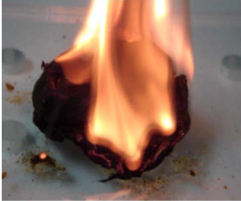
Figure 2.8: Photoignition of HiPco synthesized “fluffy” SWCNTs containing 30 wt.% Fe after 1.0 g of ferrocene was sprayed uniformly onto the cluster of nanotubes [14].
