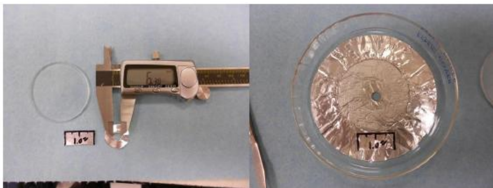
Figure 3.6: (left) Picture of precision 6.30 mm hole made in aluminum foil and placed in the (right) experimental petri dish.
