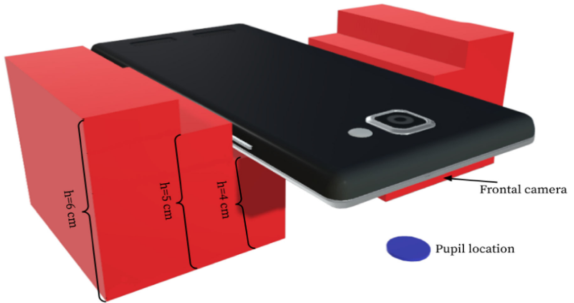
Figure 3: For distance validation, the phone is positioned at known distances above a printed image of a pupil.
