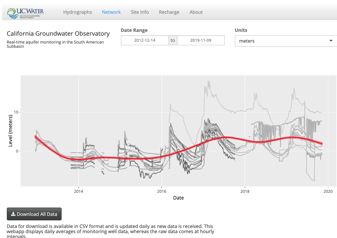
Figure 5. The network tab of the GWO shows all monitoring well data, and allows for a more complete picture of the system state. A button is provided for data download.
